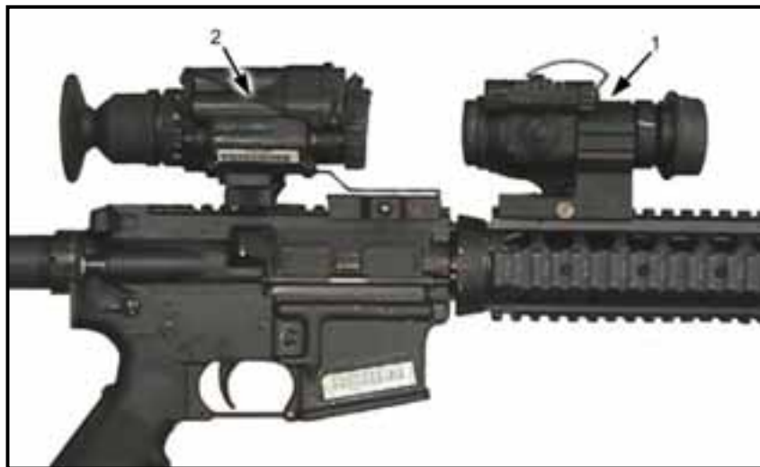
Figure 2-26. Mounting the M68/AN/PVS-14 combination on an MWS.
