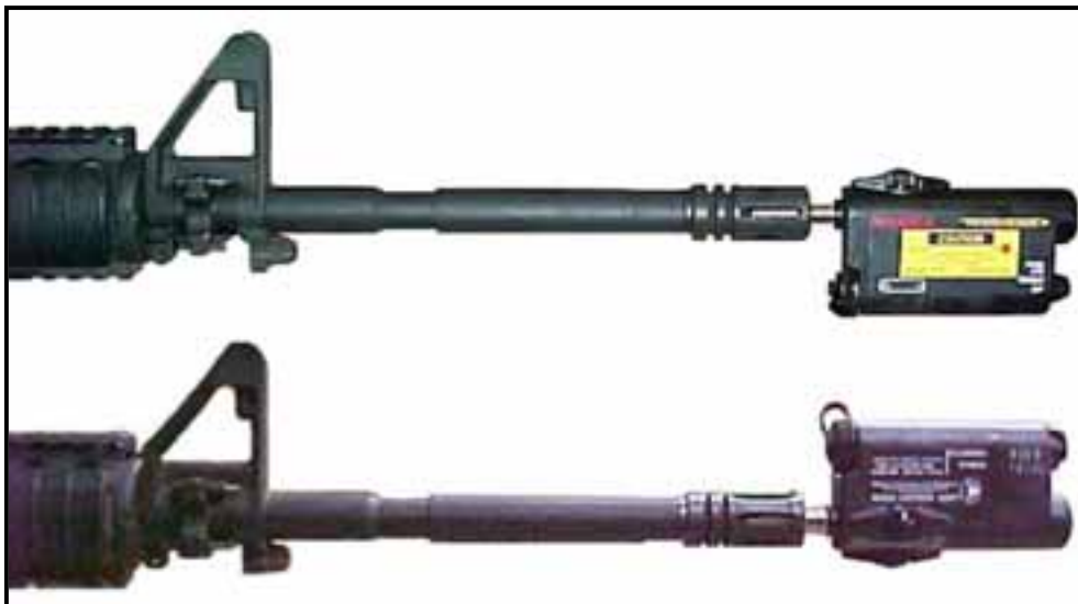
Figure 8-3. Borelight in the START POINT position.
