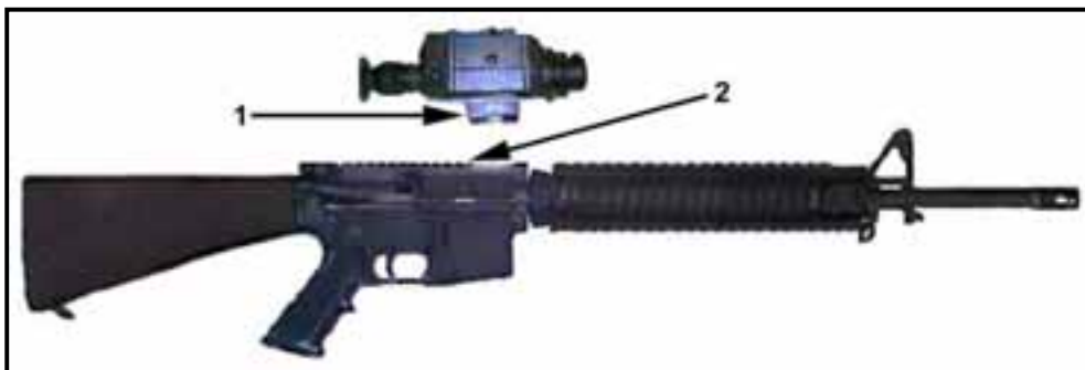
Figure 2-36. Mounting TWS on M16A4/M4-series weapons.
