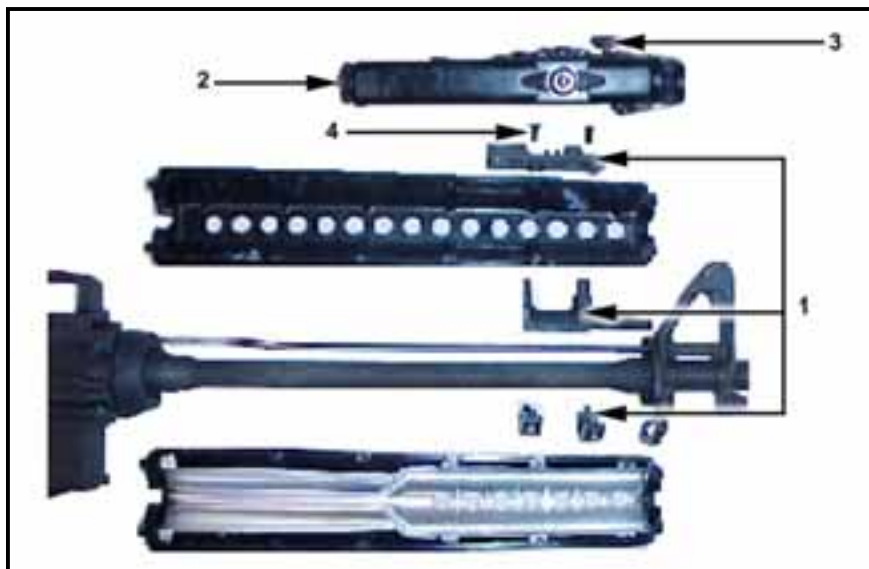
Figure 2-31. Mounting the AN/PEQ-2A to the M16A1/A2/A3 rifle and M4 carbine.
