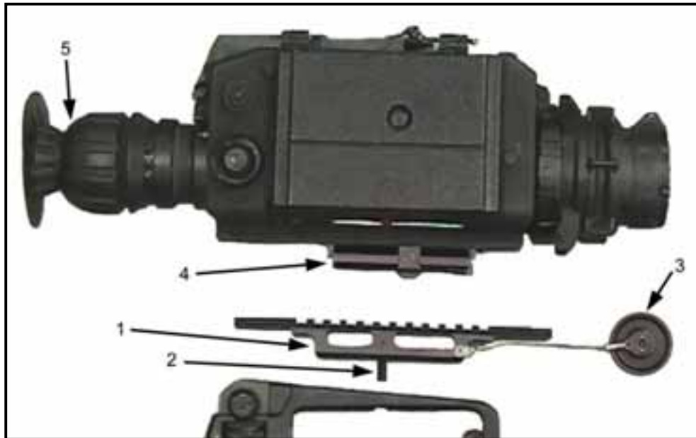
Figure 2-35. Mounting TWS on an M16A1/A2/A3.
