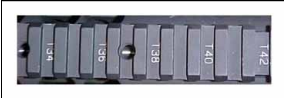
Figure 2-16. Address markings on RAS.
