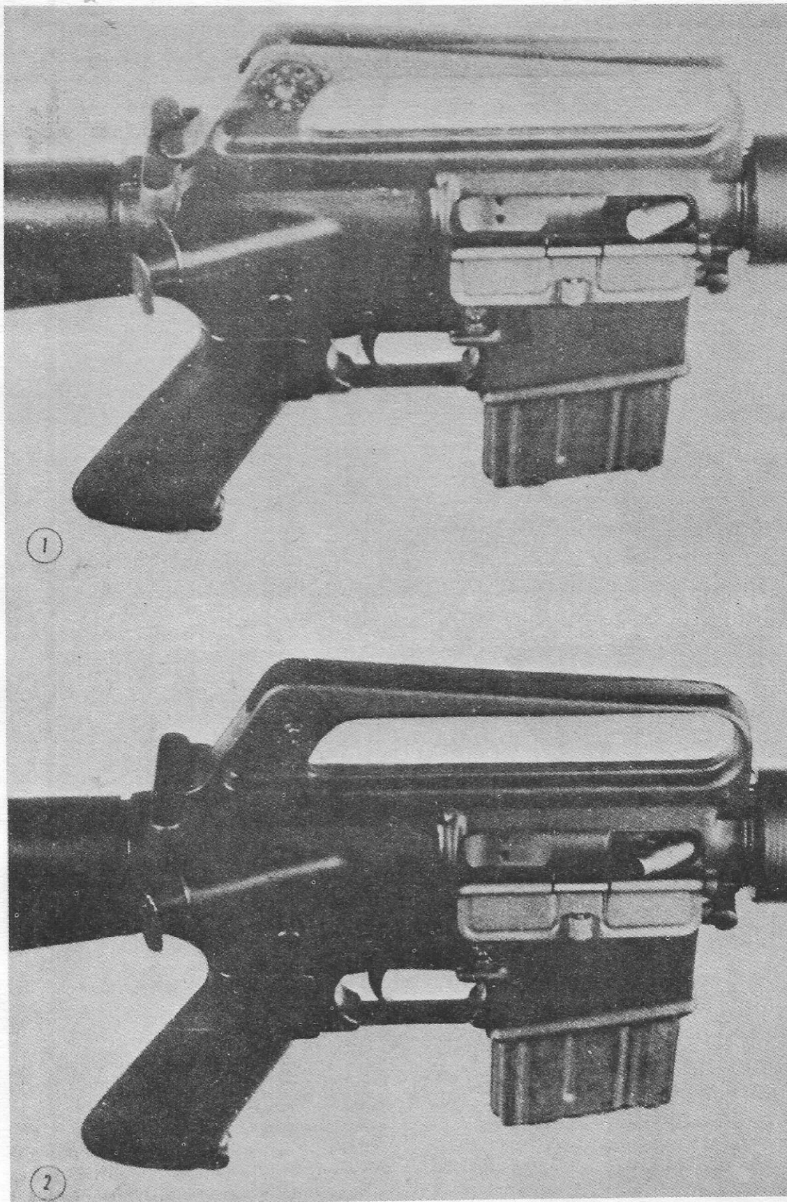
Top View—Failure-to-eject the cartridge case, base exposed. Bottom View—fired case, mouth exposed.
