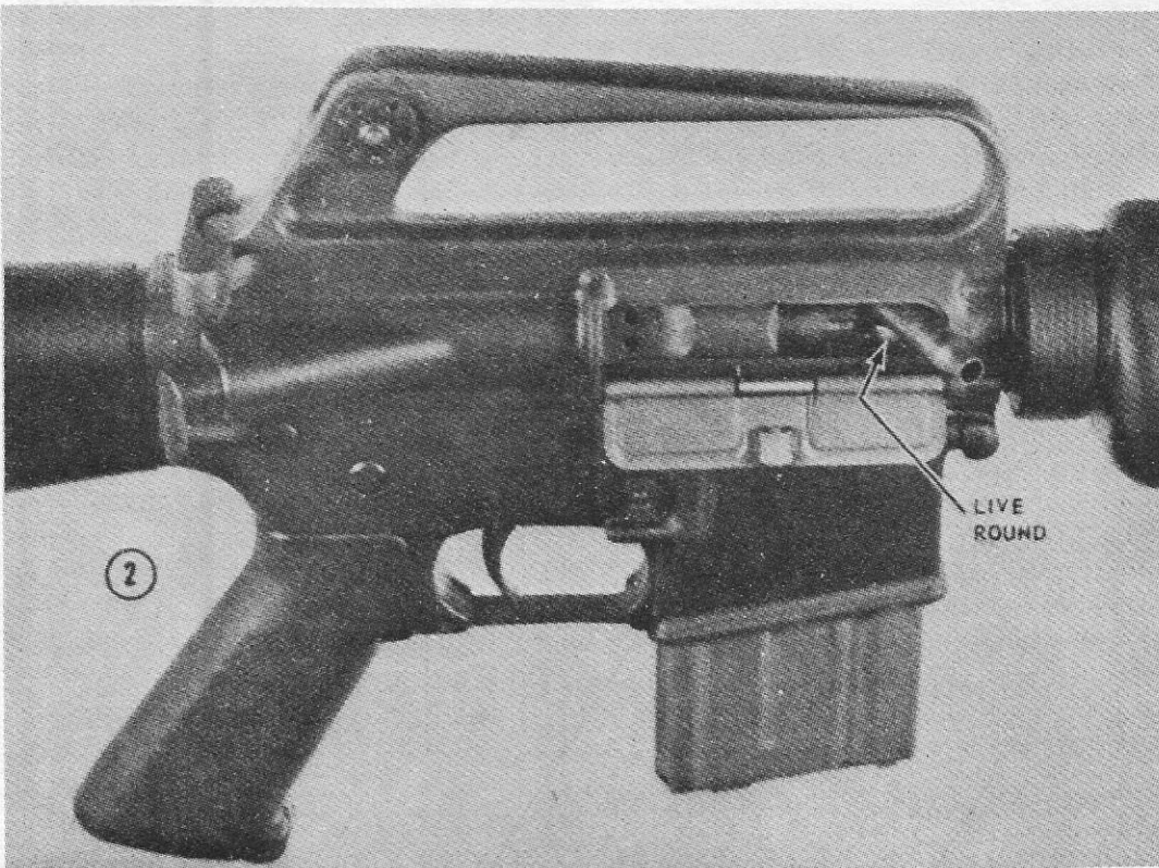
Top view—Failure-to-eject with no portion of the cartridge case outside the ejection port. Bottom view—Failure-to-eject with a live round jammed.
