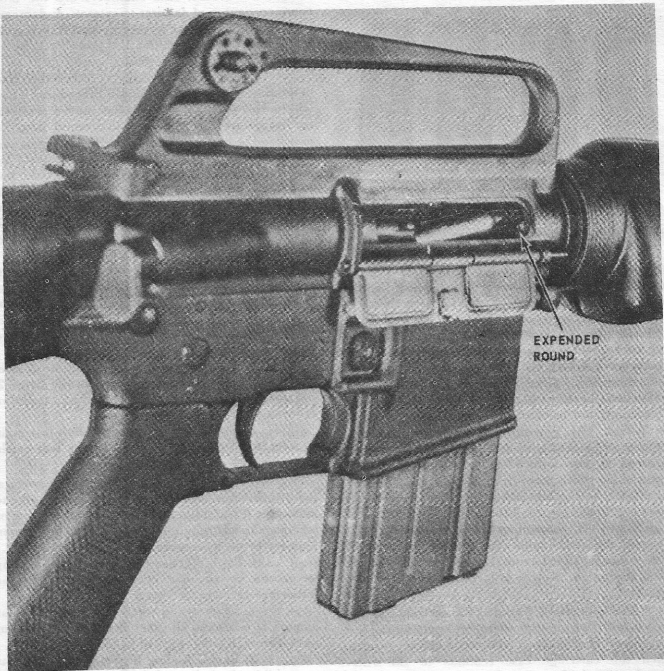
Figure 2-51. Failure-to-extract resulting in a live round being jammed against the base of the fired case.
