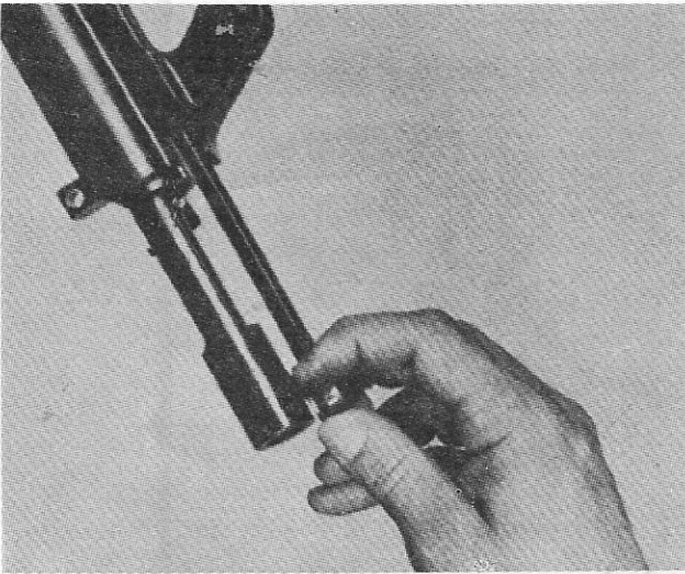
Figure 2-10. Removing charging handle and bolt carrier from upper receiver.
