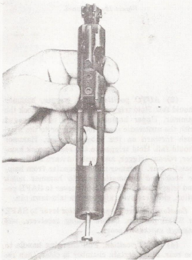
Figure 16. Removing the firing pin.
