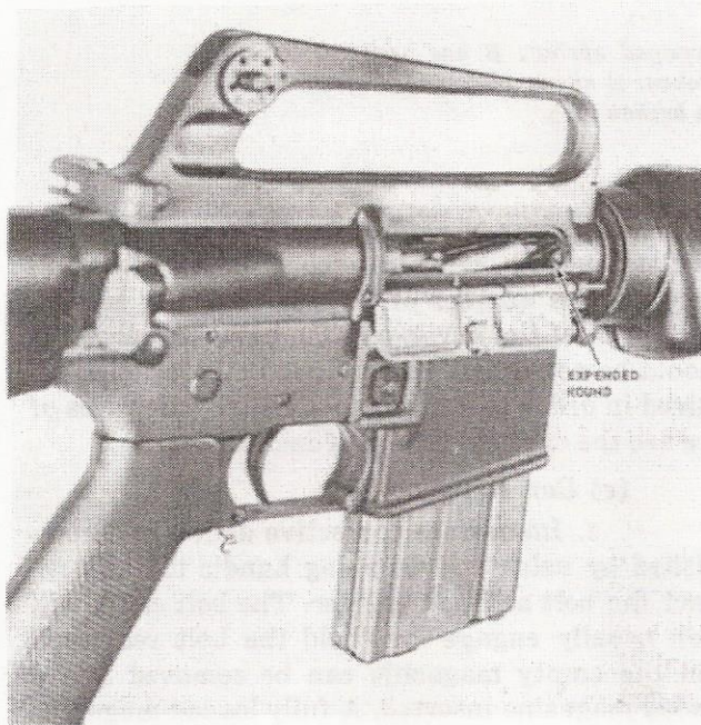
Figure 51. Failure to extract a live round jammed against the base of the fired case.
