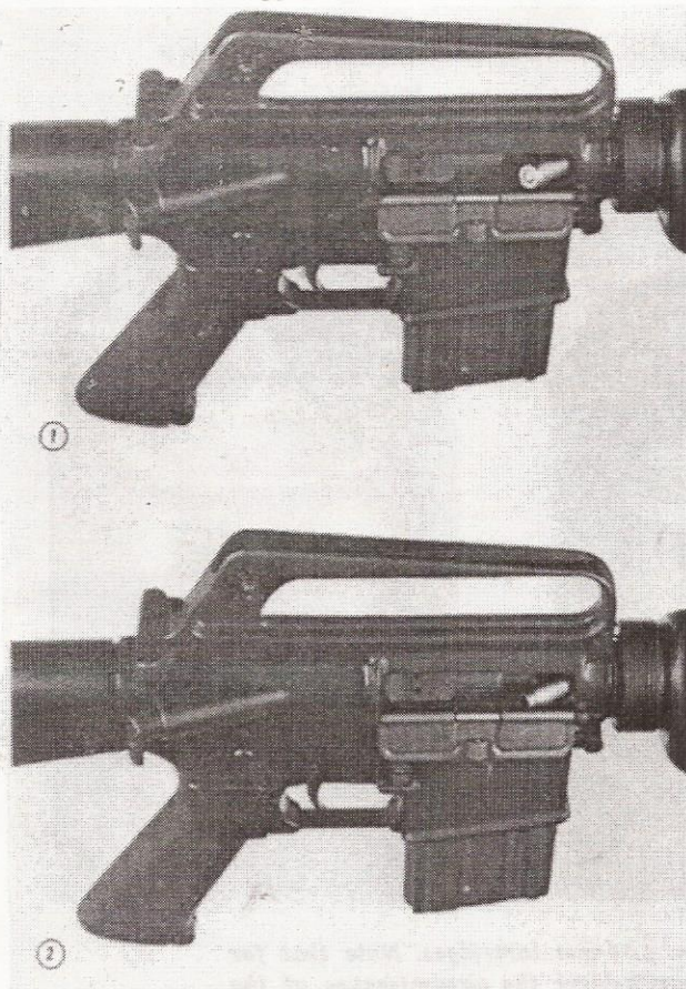
Figure 48. Two subtypes of failure-to-eject. Top—failure-to-eject the fired case, base exposed. Bottom—fired case, mouth exposed.
