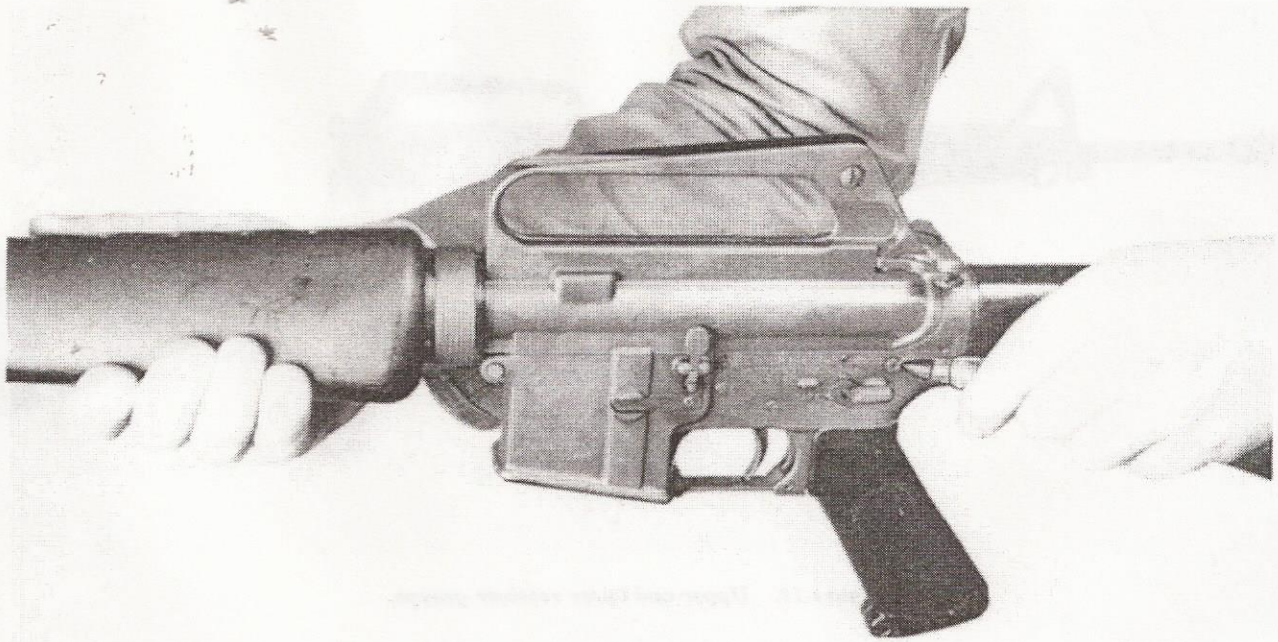
Figure 9. Pressing the takedown pin to the right.
