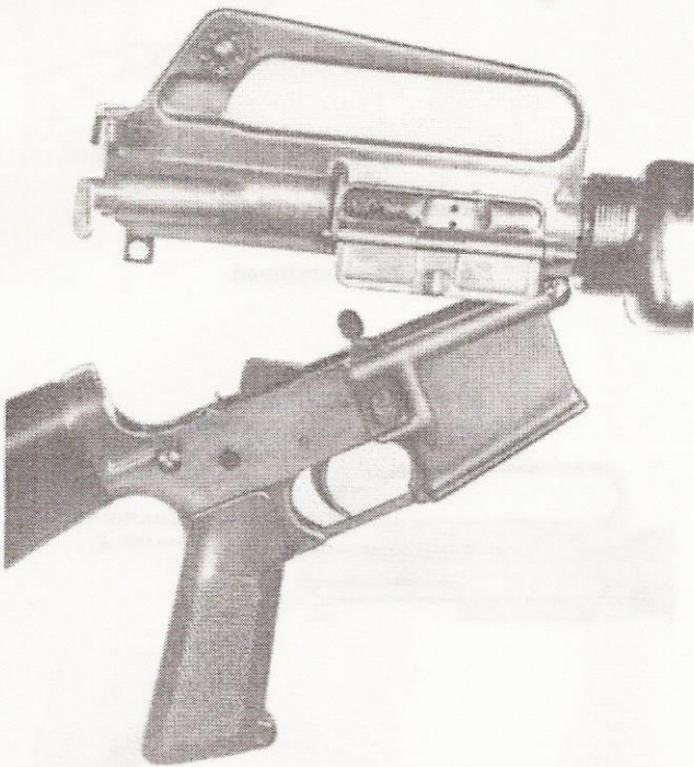
Figure 10. Breaking the upper receiver away from the lower receiver.
