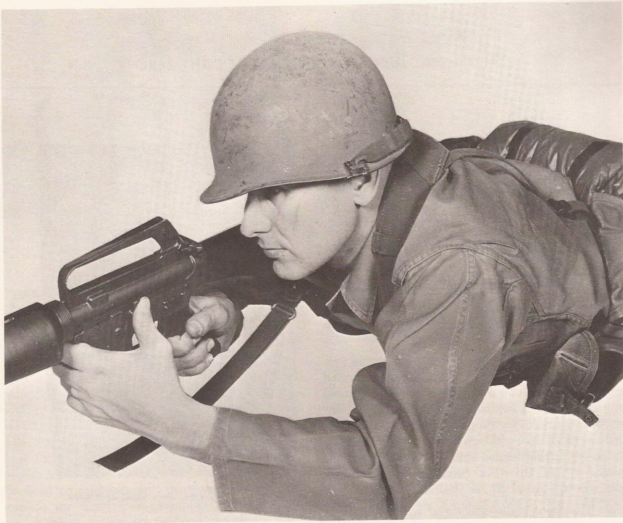
Figure 63. Releasing the bolt.
