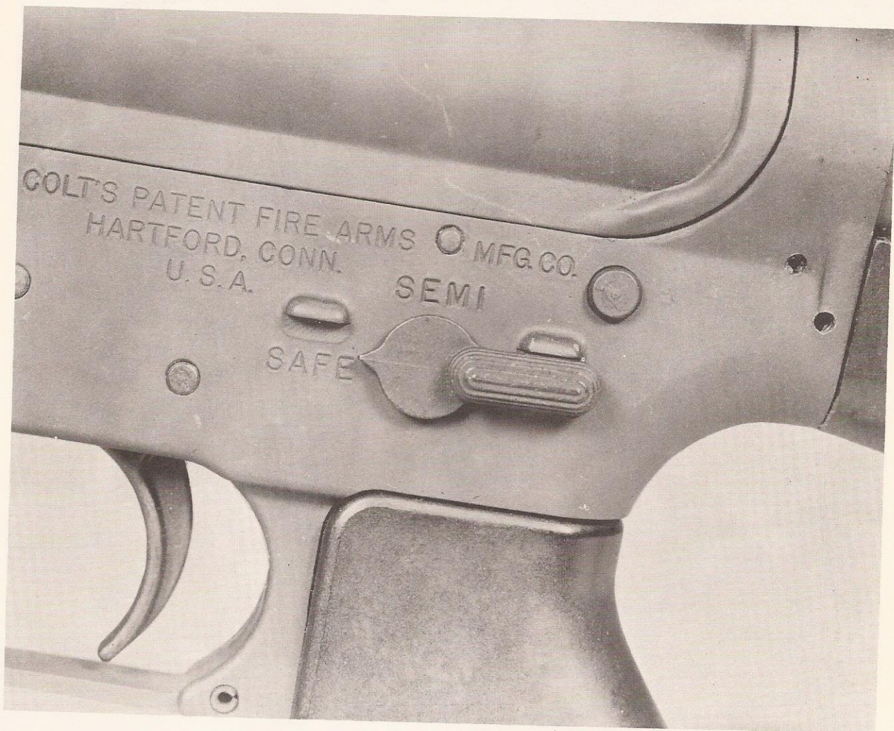
Figure 3. Selector lever pointing to SAFE.
