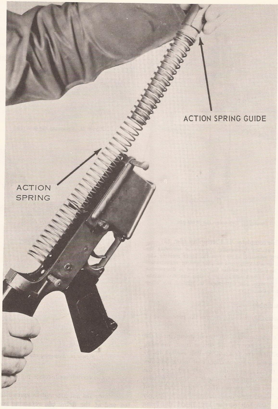
Figure 17. Removing the action spring guide assembly and action spring.
