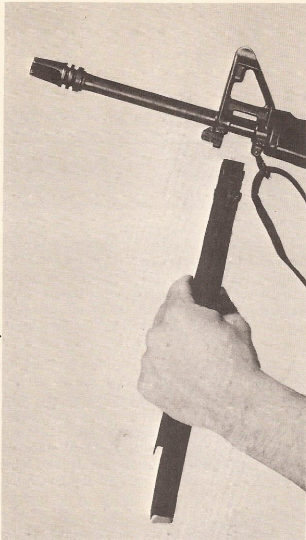
Figure 2. Attaching the bipod.
