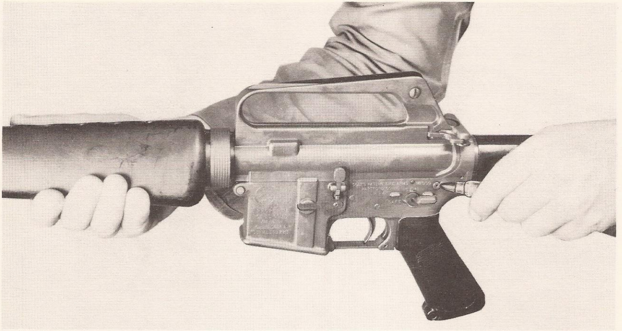
Figure 7. Pressing the takedown pin to the right.
