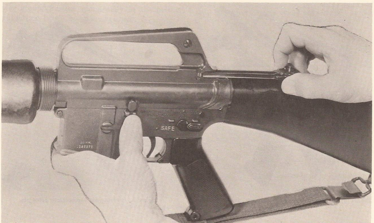
Figure 6. Locking the bolt open.
