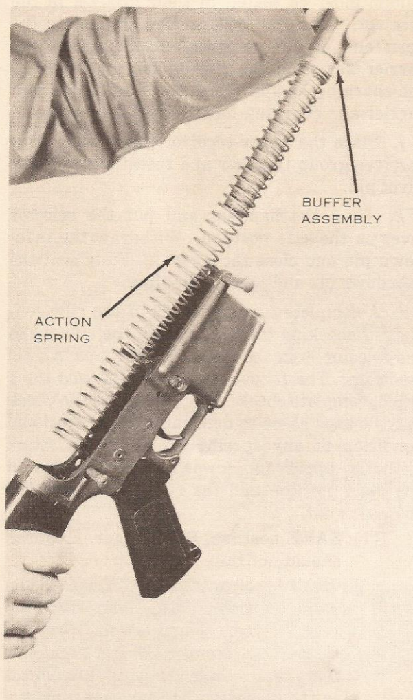
Figure 20. Removing the action spring guide assembly and action spring.
