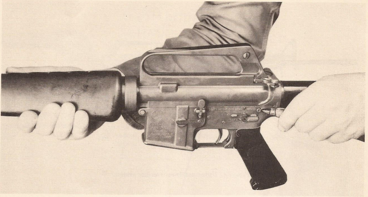
Figure 3. Pressing the takedown pin to the right.
