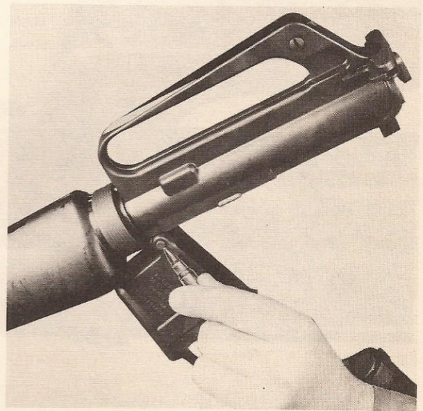
Figure 5. Pressing out the receiver pivot pin.
