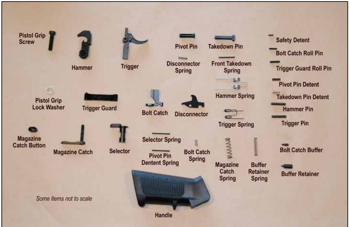
Figure 30: Lower parts kit SHOULD contain these parts. Check your kit carefully to assure you have all the parts before beginning.
