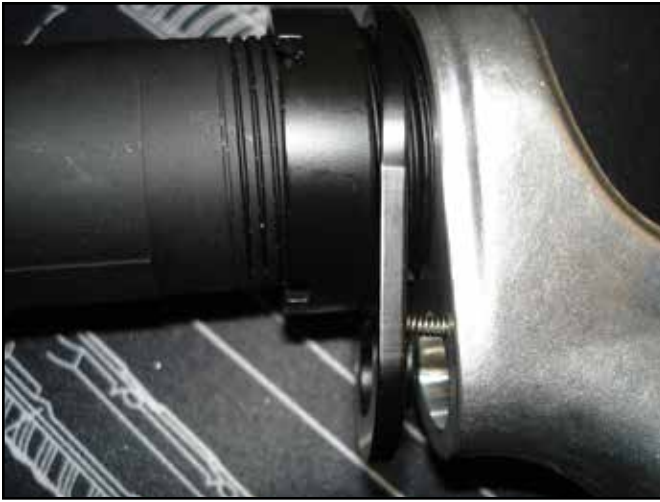
Figure 45: Castle nut installation.
