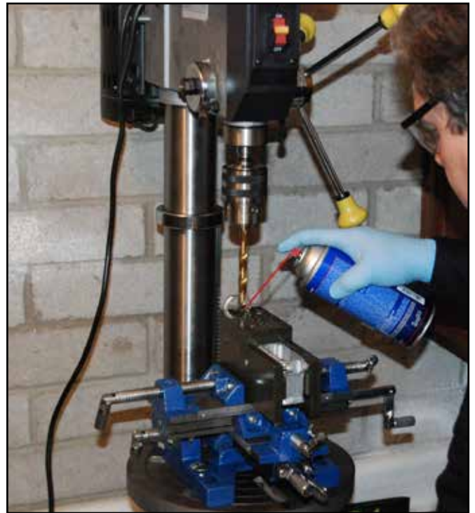
Figure 14: Drill bit in place with drilling fluid applied.
