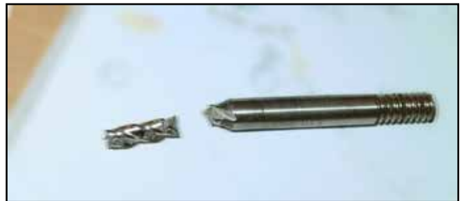
Figure 19: Snapped mill bits are more likely to occur if you rush through the process.
