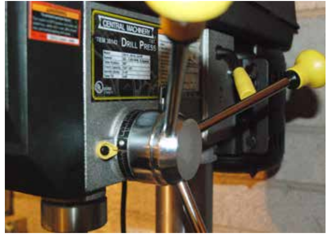
Figure 11: Depth stop collar will help prevent drilling too deep.
