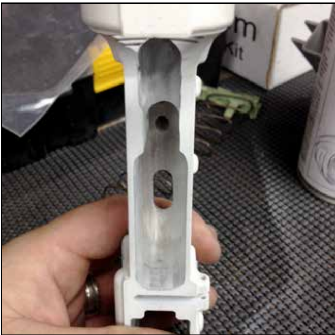
Figure 25: Finished fire control pocket.
