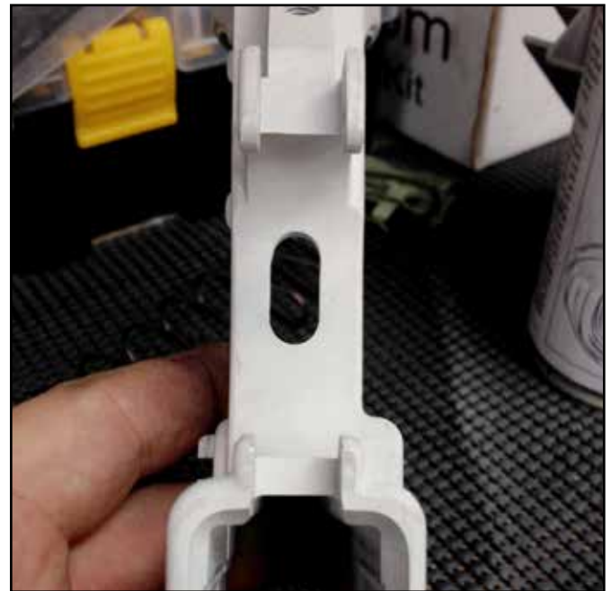
Figure 26: Bottom view of finished fire control pocket.
