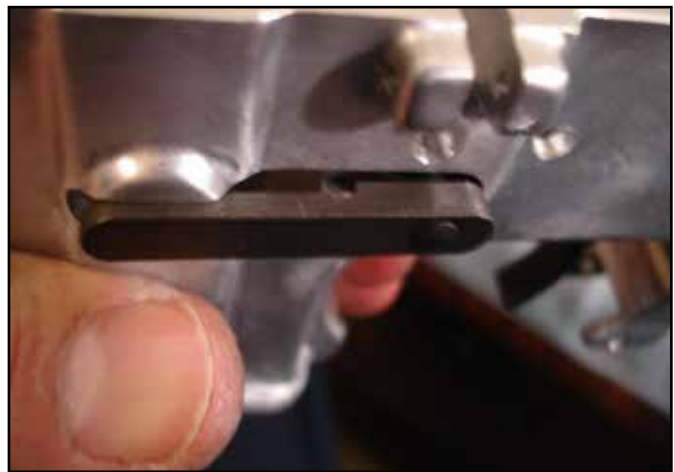
Figure 33: Magazine catch installation.
