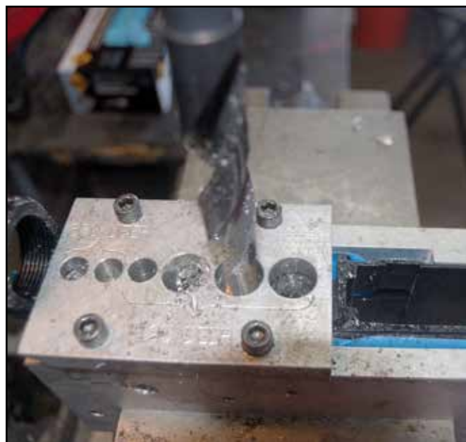
Figure 16: You will need to remove the excess debris from the receiver quite often to avoid bogging down the bit.
