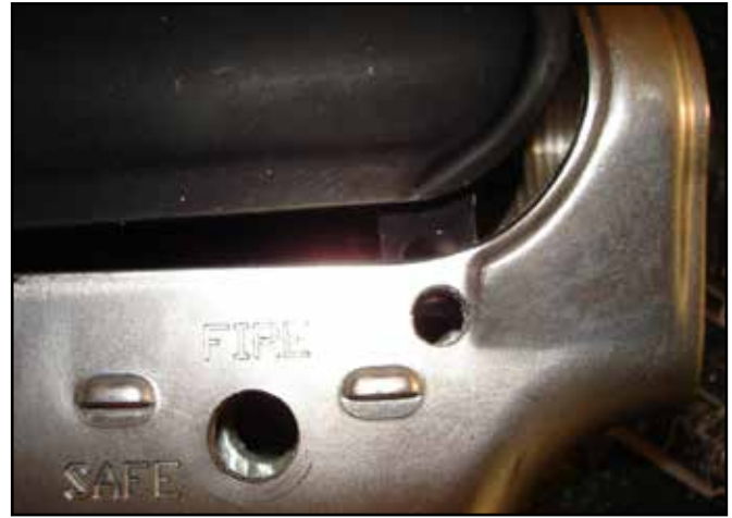
Figure 53: Check the fit of the upper and lower receivers to determine how much more is necessary to sand or grind.
