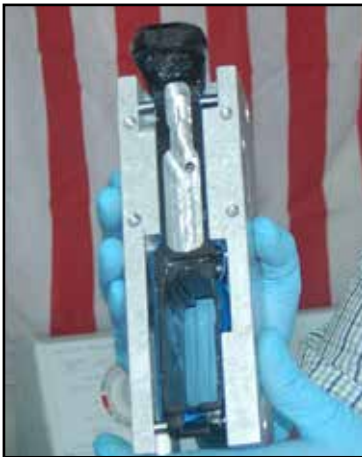
Figure 21: The milling plate allows you to continue to mill the deeper section of the fire control pocket.
