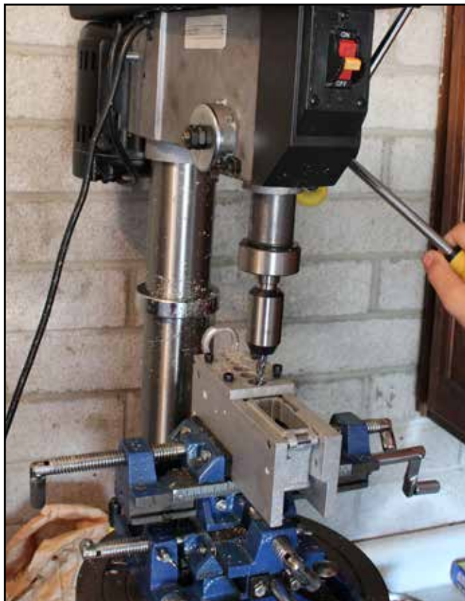
Figure 15: Drill slowly and carefully the first set of holes.
