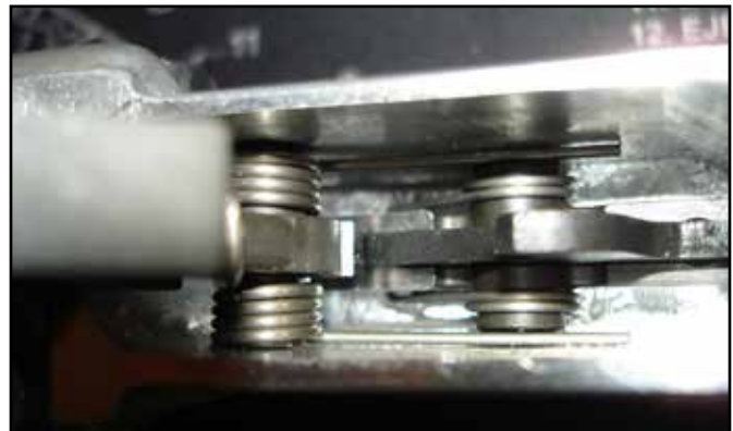
Figure 41: Hammer assembly installed.
