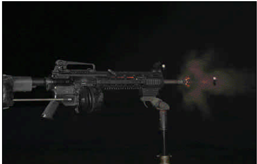
Above: The gas tube can be seen glowing bright red while 3 cases are suspended in the air and an almost perfect star-burst leaves the muzzle. This rifle, a standard direct gas impingement version faced the same heavy usage as the P-416 but could not complete the test due to a gas tube failure early into the testing.
