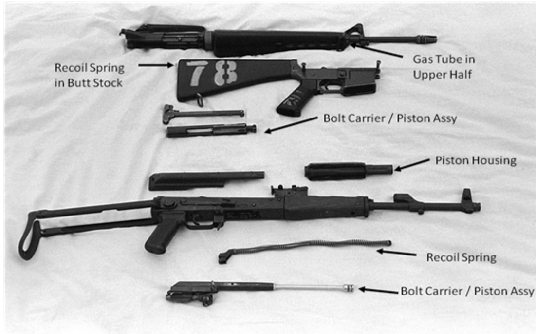
Figure 1: A United States M-16A1 rifle (top) compared to a Soviet Union AK rifle (bottom). The two rifles are disassembled into groups. (3)
