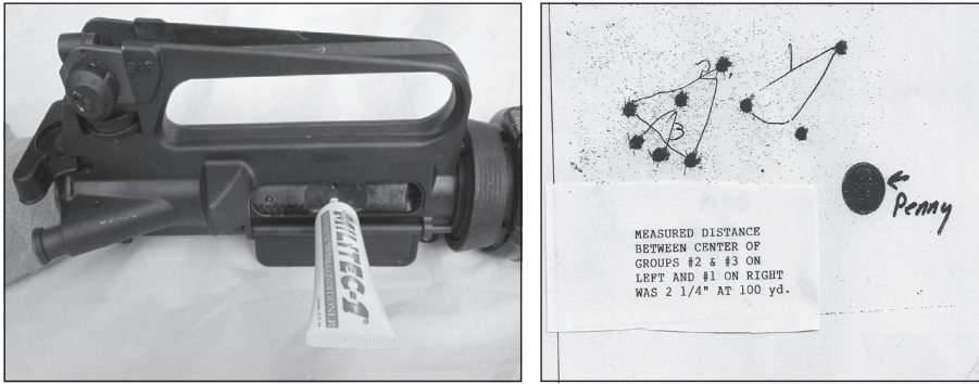
Above left: Adding oil during range sessions or when testing magazines will help insure consistency in bolt carrier velocity and points of impact. Above right: This magazine test scan shows 2.25" distance between group centers.
