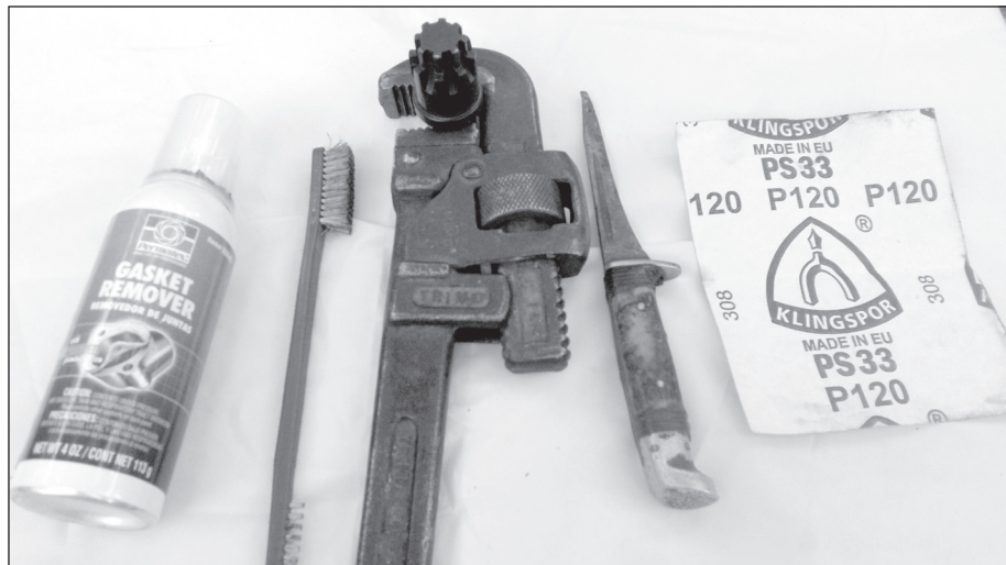
Above: Recommended clean up tools and supplies: Barrel extension tool (center) with gasket remover and metal gunsmith's tooth brush on left and old knife and either fine emery paper or steel wool on right.
