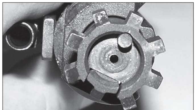
Below left: The carrier key at the bottom is properly staked the one at the top is not. This is trouble waiting to happen. Below right: Check the bolt ejector and extractor closely. These can be real trouble spots.
