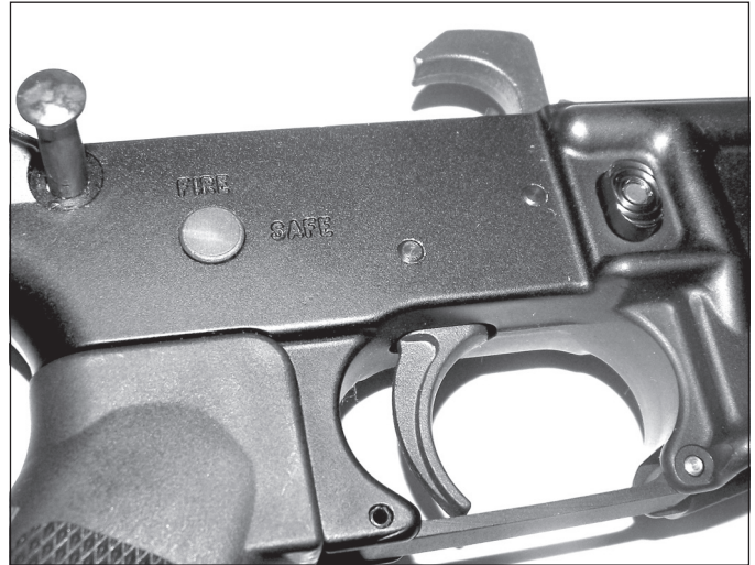
Above left: The carrier key must be properly staked or the rifle is subject to serious malfunction. Above right: The action pins must be tight and flush with the receiver or trouble is looming.
