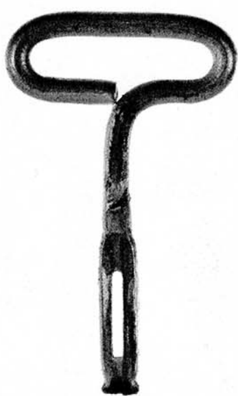
Figure 2, 6473/66: Keys Broke at 0° and 155°F Firings.
