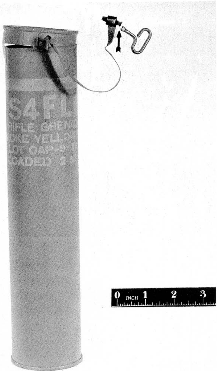
Figure 1, 6476/66: Metal Grenade Container Opened with Pliers due to Broken Key.
