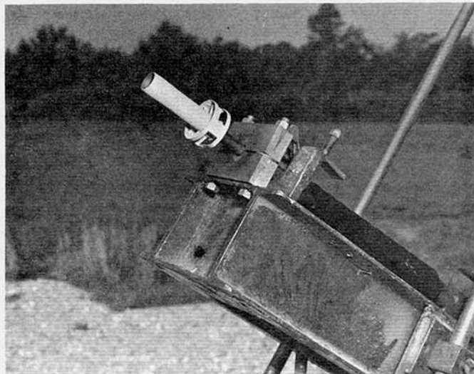
Figure 2 (U): Stabilizer That Remained on Rifle Fitted with Maximum Size Flash Suppressor. Grenade and Base Impacted 75 Yards Forward of the Gun Position (U).
