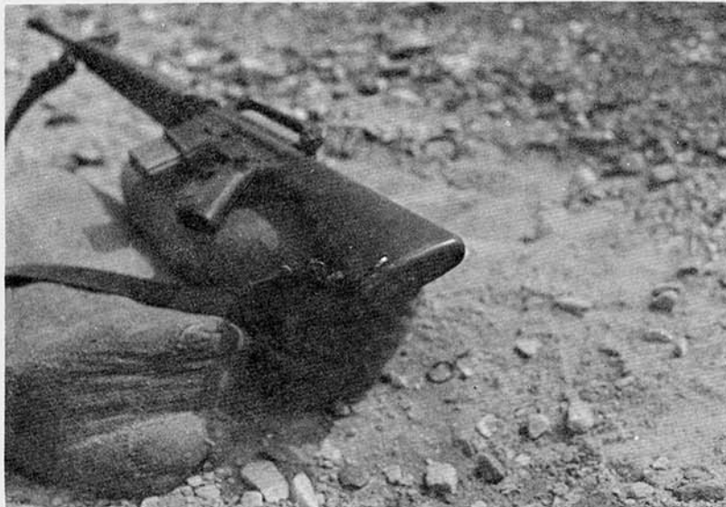
Figure 8 (U): Left Side of Stock on Rifle Fitted with the Maximum Flash Suppressor upon Completion of Firings from the Kneeling Position (U).
