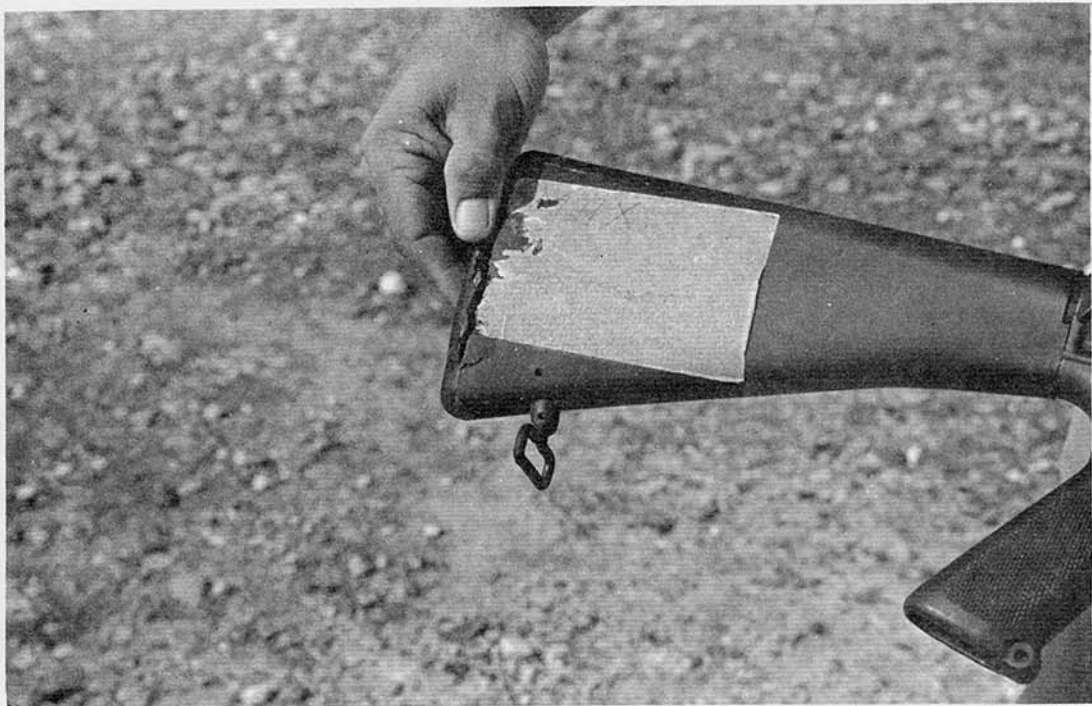
Figure 6 (U): Right Side of Stock on the Rifle Fitted with Maximum Flash Suppressor upon Completion of Test Stand Firings (30 Rounds) (U).
