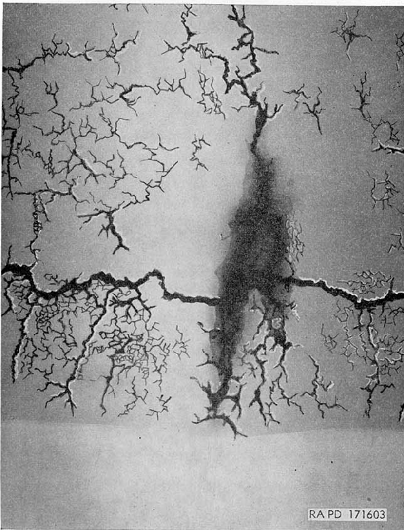
Figure 42. Severe liner rupture, cal..50 machine gun.
