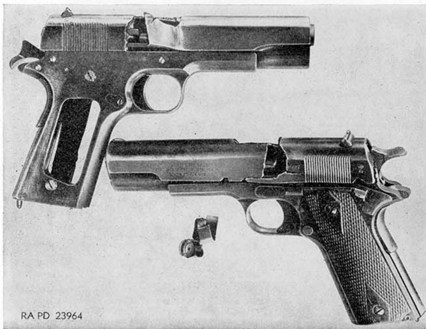
Figure 8. Damage from firing round with double charge of powder, cal..45 automatic pistol M1911.
