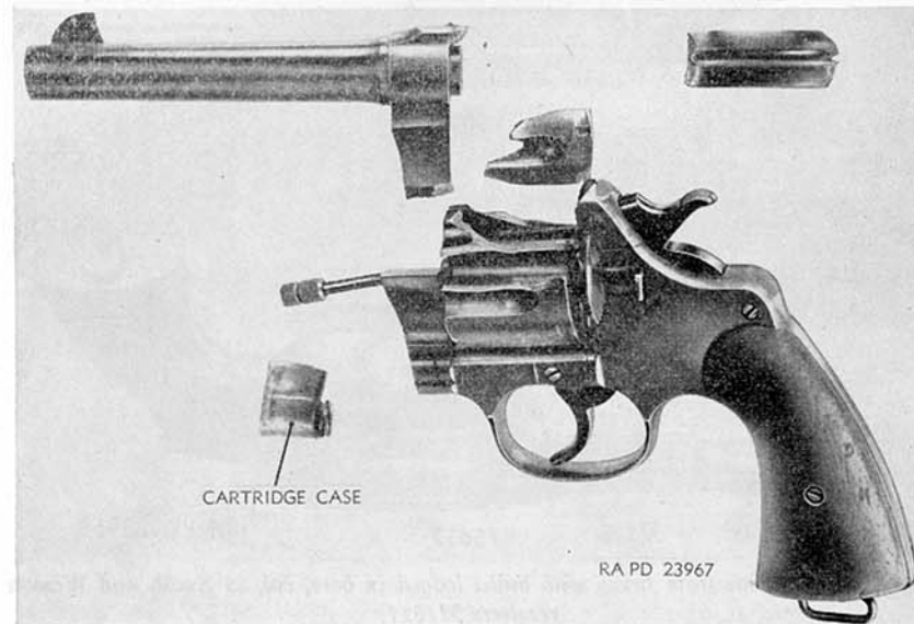
Figure 1. Damage from firing round with double charge of powder, cal..45 colt revolver M1917.
