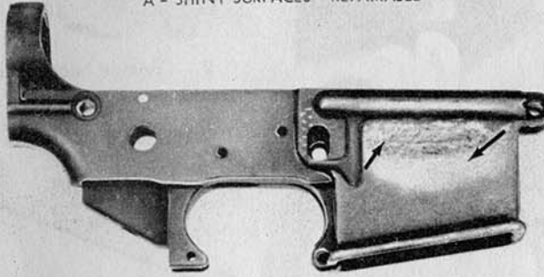
B - CORRODED AND NO HOLES - REPAIRABLE
