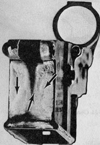
B - CORRODED - REPAIRABLE
