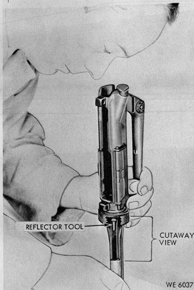
Figure 3-13. Visually inspecting the chamber using reflector tool.
