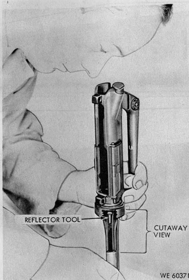
Figure 3-13. Visually inspecting the chamber using reflector tool.
