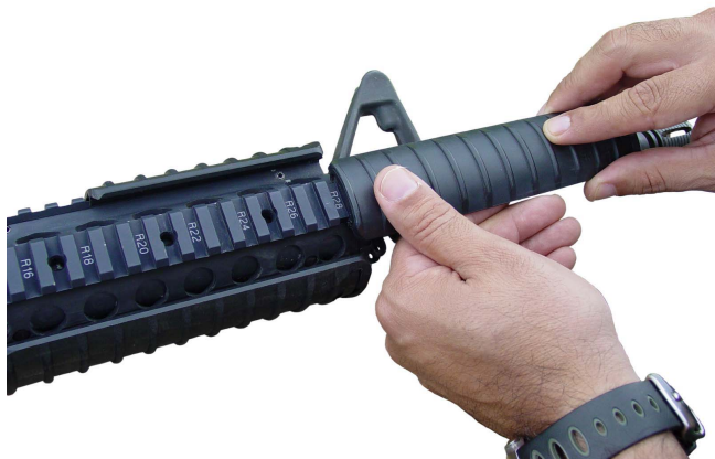
Figure 1-7. Installation of Handguard Sections to RAS
