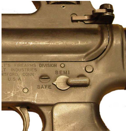
Figure 2-7. Selector lever - SAFE
