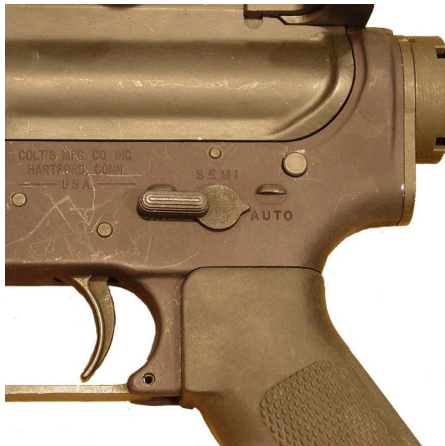
Figure 2-10. M4A1 CQBW Only - Selector lever - AUTO
