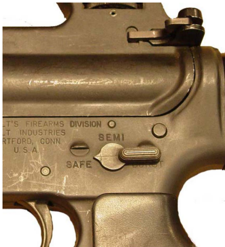
Figure 2-22. Selector lever - SAFE
