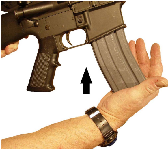
Figure 2-13. Seating the Magazine
