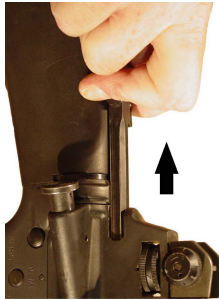
Figure 2-39. Pull Charging Handle
