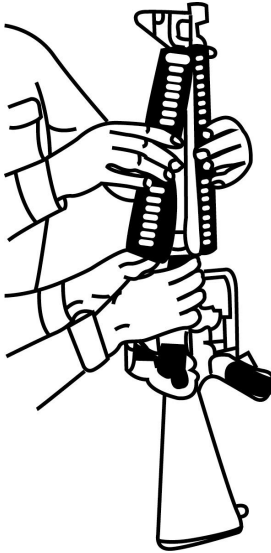
Figure 3-1. Removing Handguards Using the “Buddy System”
