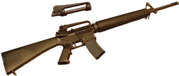
Figure 1-2. M16A4 with Removable Carrying Handle
