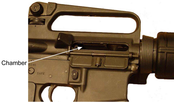
Figure 2-25. Checking Chamber for Ammunition
