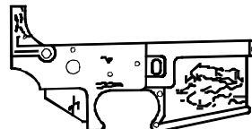
CORRODED AND NO HOLES (REPARABLE)
