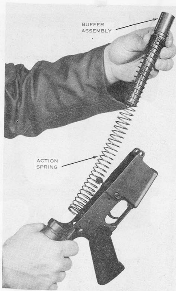
Figure 19. Removing the action spring guide assembly and action spring.
