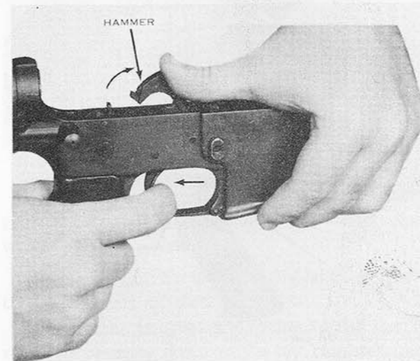
Figure 16. Lowering the hammer.
