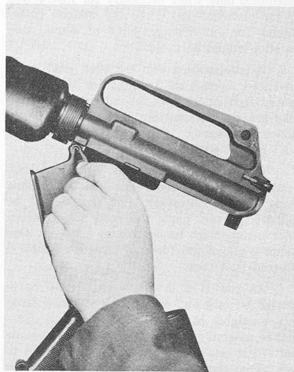
Figure 5. Pressing out the receiver pivot pin.
