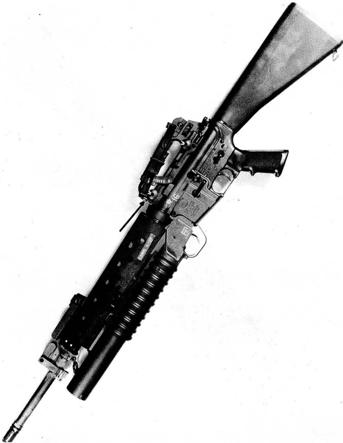
Figure 6. Showing left side view of Enhanced M16A2 rifle with M203 grenade launcher attached. The full range launcher sight, mounted on the carrying handle/rear sight assembly is set at 150 meter range. At this point the launcher sight contacts the front clamp screw nut and prevents sight travel to maximum range (400 meters).
