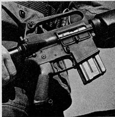
U.S. Rifle M16A1, Caliber 5.56mm (note bolt closure push rod)
