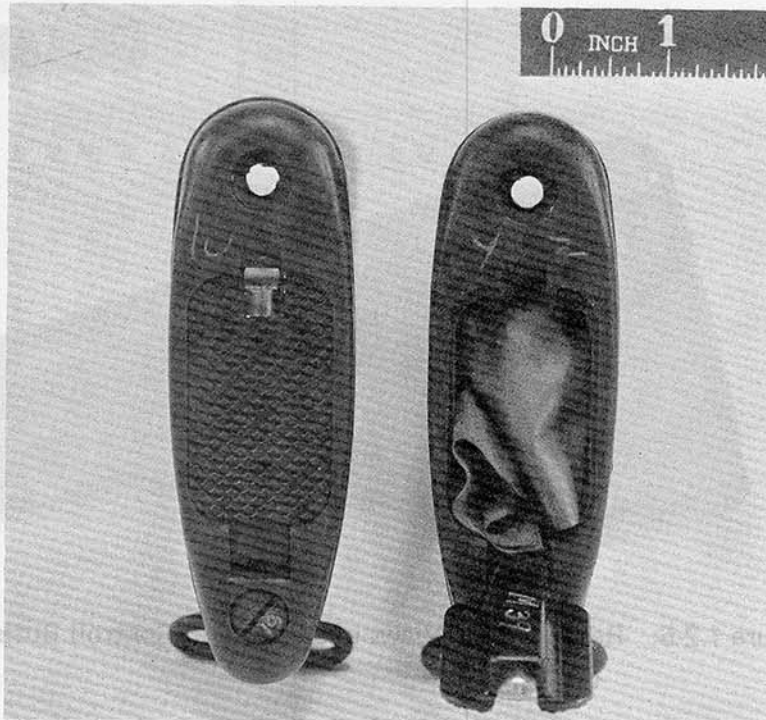
Figure 1.2-3: Rear View of Modified Buttstock with Trap Door Assembly. LEFT: Closed Position. RIGHT: Open Position with Cleaning Package Kit in Place.
