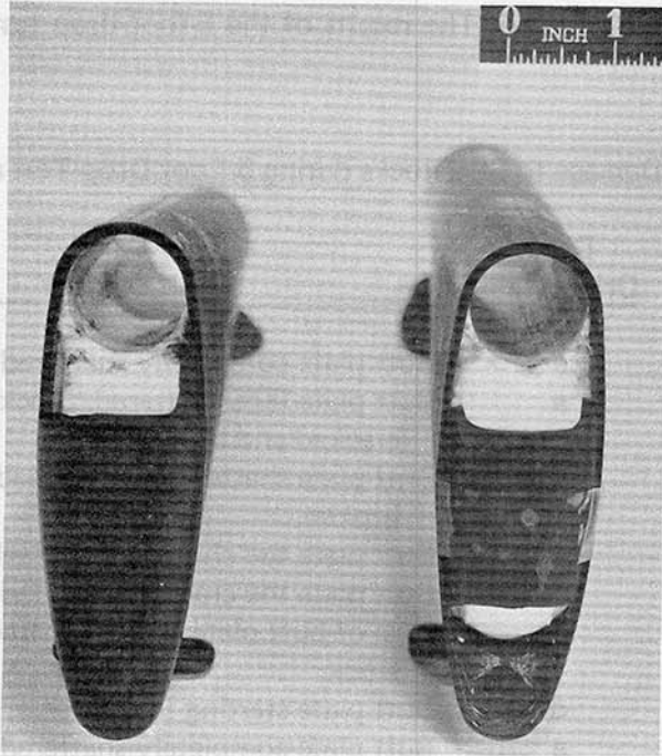
Figure 2.4-1: LEFT: Control Buttstock No. 8 after 25 Rifle Grenade Firings. RIGHT: Control Buttstock No. 10 after 37 Rifle Grenade Firings Made in the Low-Temperature Test (-65°F).
