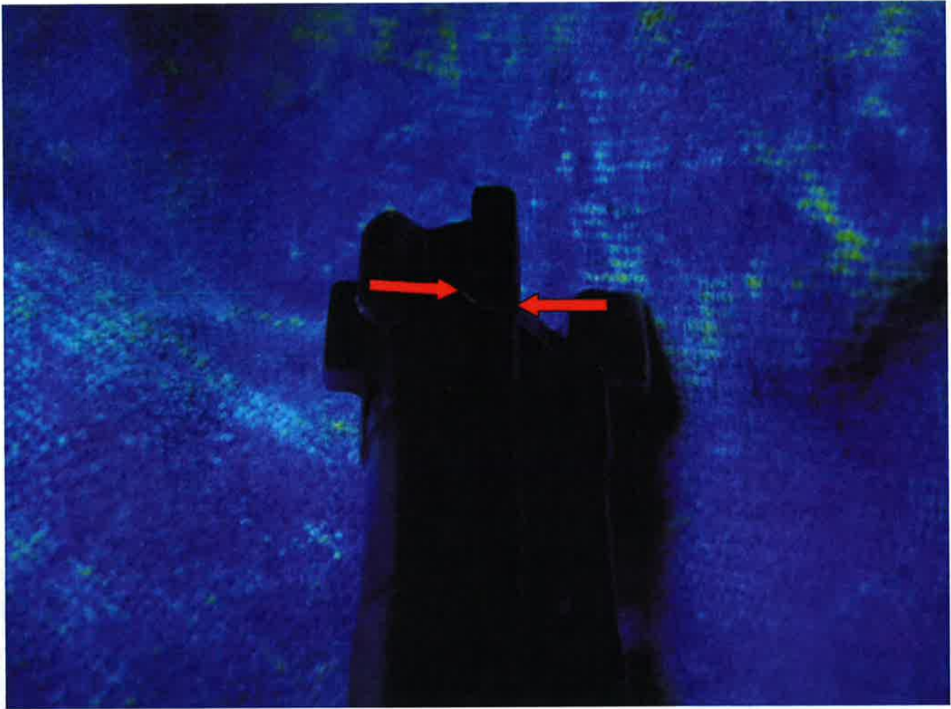
Figure 2. M27, 5.56mm, SN. 172-003777. The arrows show a 3mm indication indicative of a crack pattern forming on a bolt lug.
