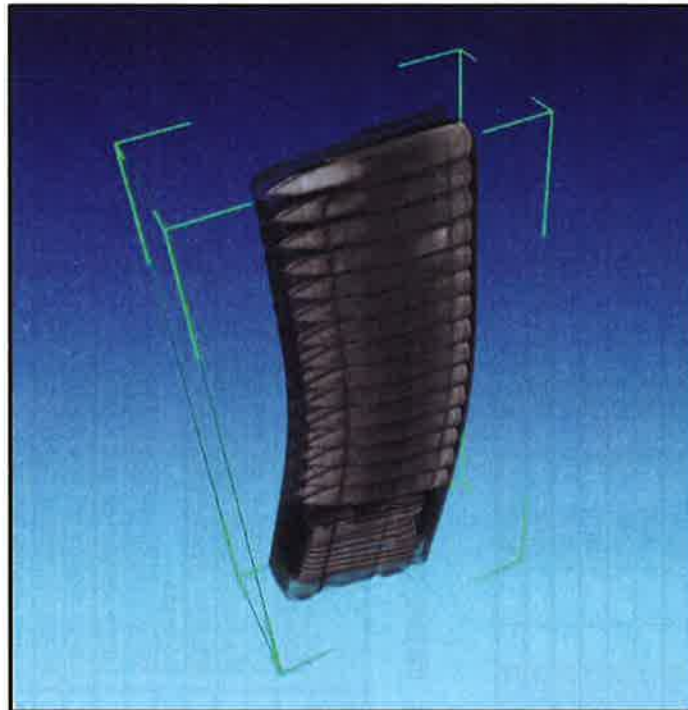
Figure 2.1-3. CT X-ray standard magazine.
