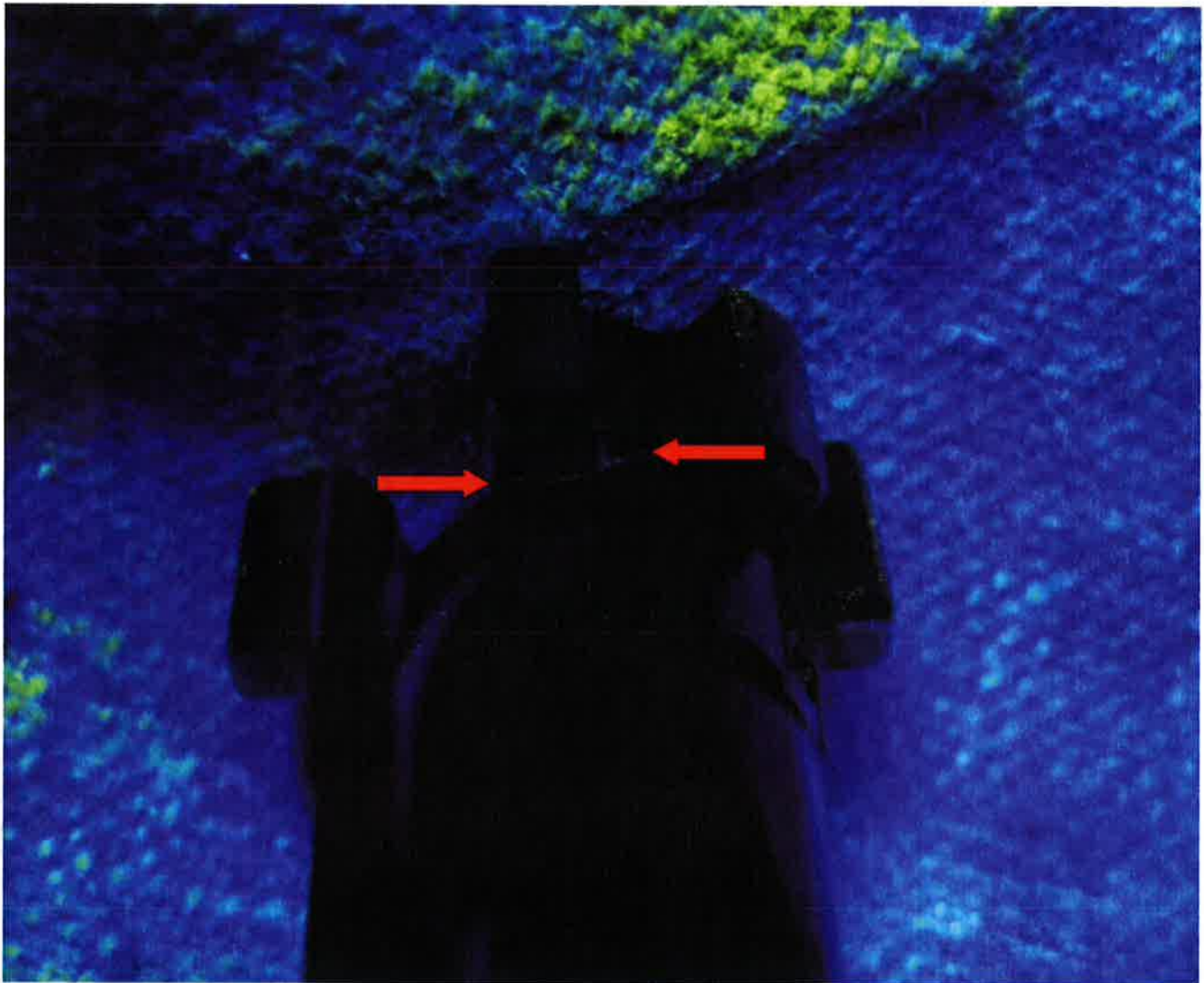
Figure 1. M4A1, 5.56mm, SN. W499818. The arrows show a 5mm indication indicative of a crack pattern forming on a bolt lug.
