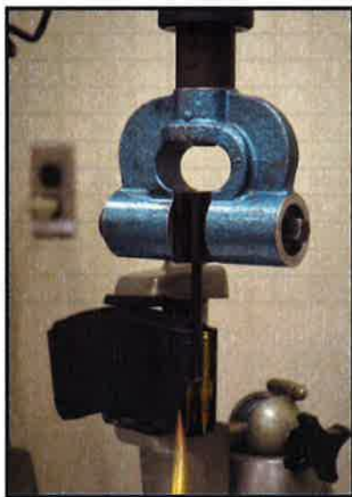
Figure 2.1-2. Magazine being unloaded by an Instron machine.
