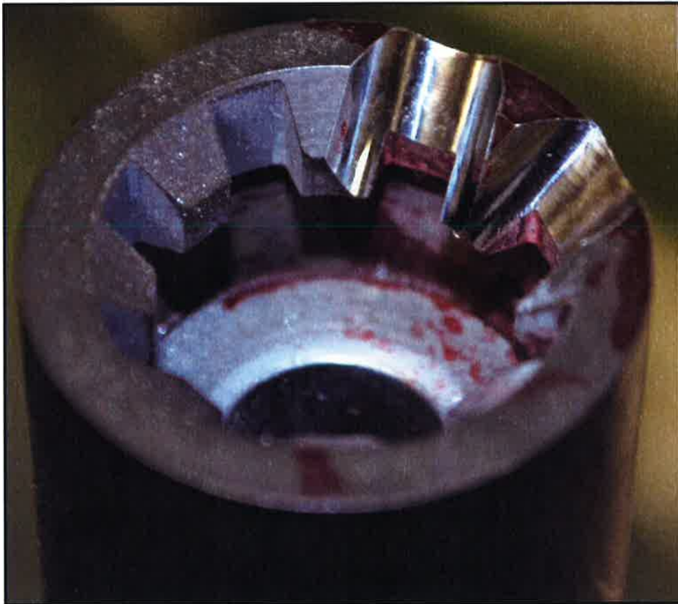
Figure 2.3-1. The barrel extension and barrel with the (b) machined feed ramps.
