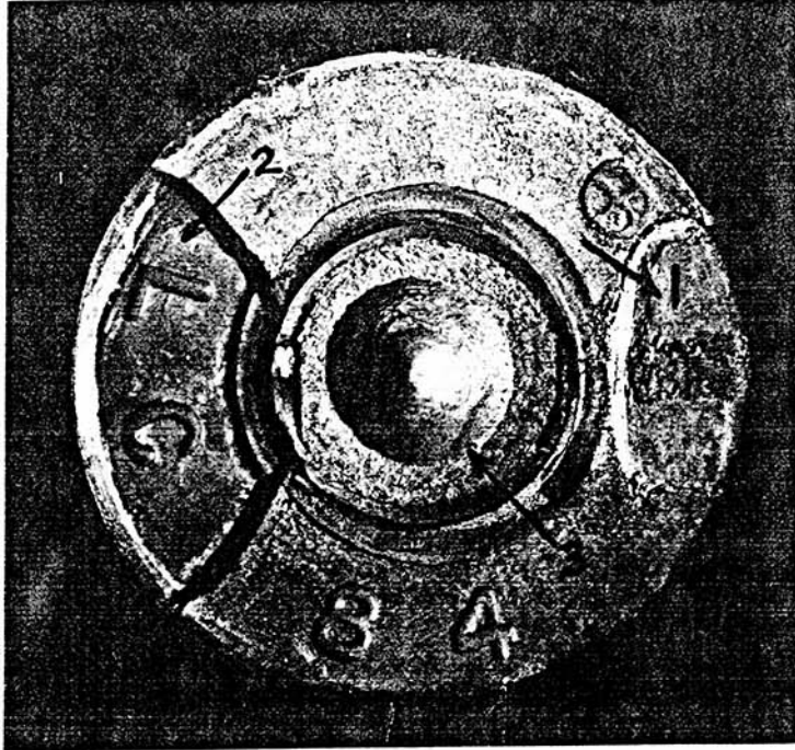
Figure 5.8-1. Typical cook-off round fired case from an M249 SAW showing heavy set back into bolt face (arrow 1 and 2) and protruding primer (arrow 3).
