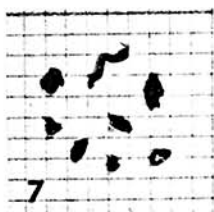
Figure 5.10-2. Recovered particles ejected from CONUS produced M856 tracer projectiles during firing at 10-meter range. Note: Grid scale = 0.1 inch.
