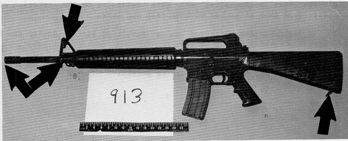
Figure 9-3. Rust condition of M16A2 rifle No. 913 after 48-hour salt fog environment. The arrows indicate the location of rust on the M16A2 rifle after 48 hours in a salt fog environment.
