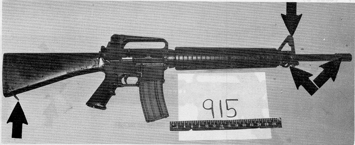
Figure 9-4. Rust condition of M16A2 rifle No.915 after 48-hour salt fog environment. The arrows indicate the location of rust on the M16A2 rifle after 48-hours in a salt fog environment.
