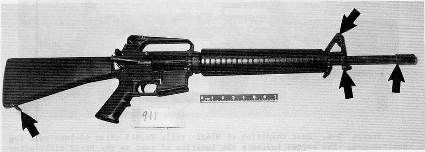
Figure 9-6. Rust condition of M16A2 rifle No. 911 after a 48-hour drying period. The arrows indicate the location of rust discovered after 48 hours of drying after being subjected to a 48-hour salt fog environment.
