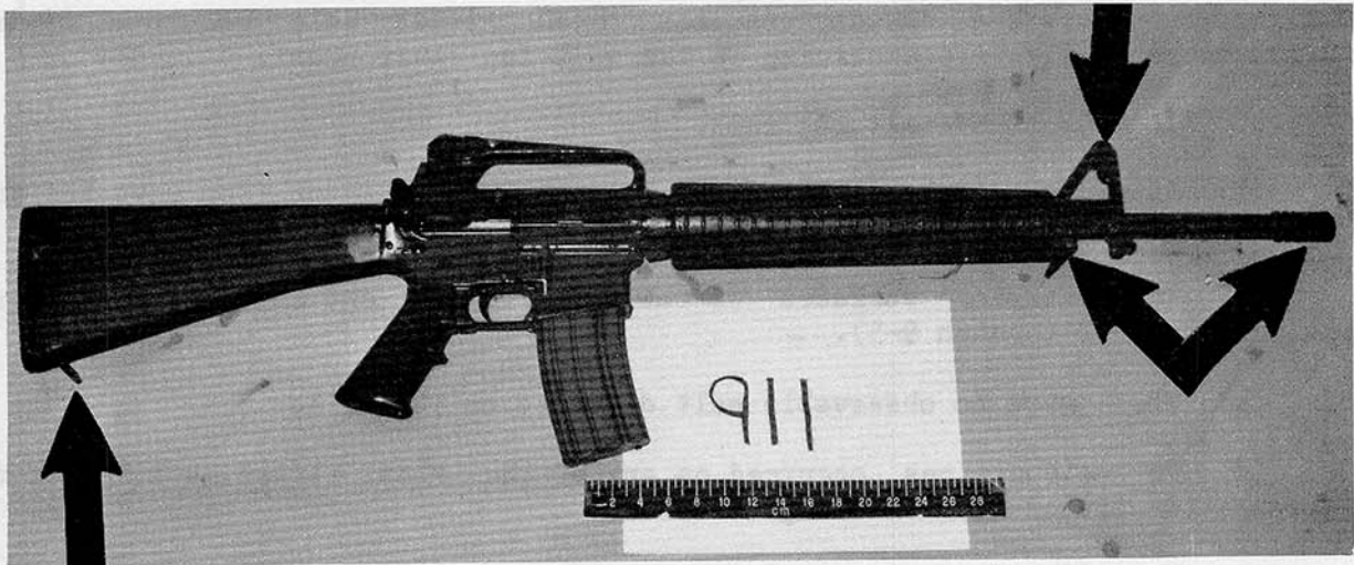
Figure 9-2. Rust condition of M16A2 rifle No. 911 after 48-hour salt fog environment. The arrows indicate the location of rust on the M16A2 rifle after 48 hours in a salt fog environment.
