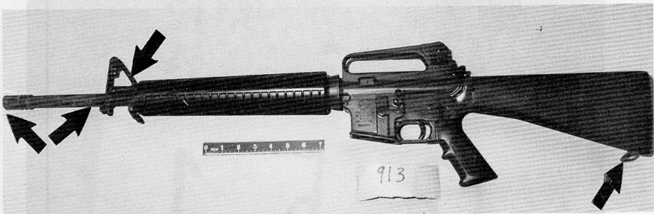
Figure 9-7. Rust condition of M16A2 rifle No. 913 after 48-hour drying period. The arrows indicate the location of rust discovered after 48 hours of drying after being subjected to a 48-hour salt fog environment.
