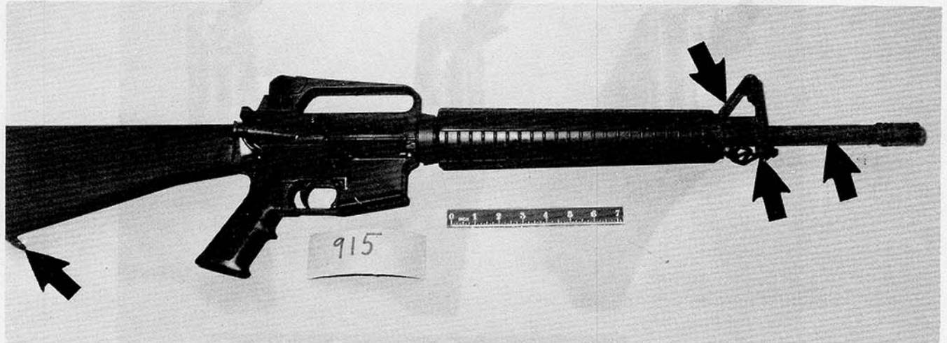
Figure 9-8. Rust condition of M16A2 rifle No. 915 after 48-hour drying period. The arrows indicate the location of rust discovered after 48 hours of drying after being subjected to a 48-hour salt fog environment.
