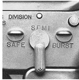
Full automatic with Model 701. Three-shot burst control with Model 705.
