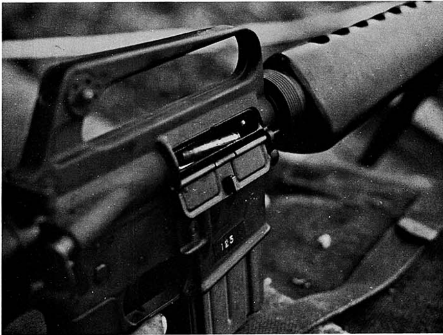
FIGURE C15a. Spent Cartridge Reentering Upper Receiver After Rebounding from Rear Edge of Ejection Port
