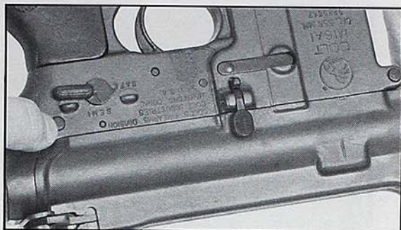
STEP 1. PUSH TAKE-DOWN PIN TO START.
