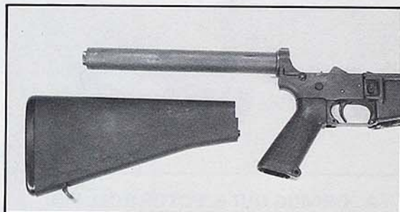
D. BUTTSTOCK REMOVED.
