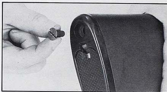
B. BUTT CAP SCREW REMOVED.
