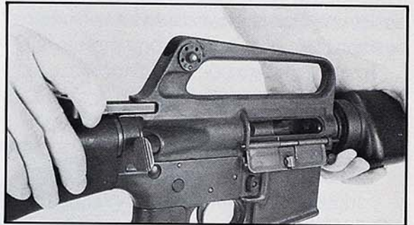
STEP 2. PULL CHARGING HANDLE BACK AND INSPECT CHAMBER.
