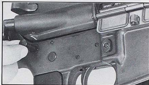
STEP 2. PULL TAKE-DOWN PIN OUT TO DETENT.
