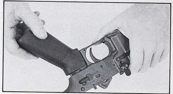
B. PISTOL GRIP REMOVAL.
