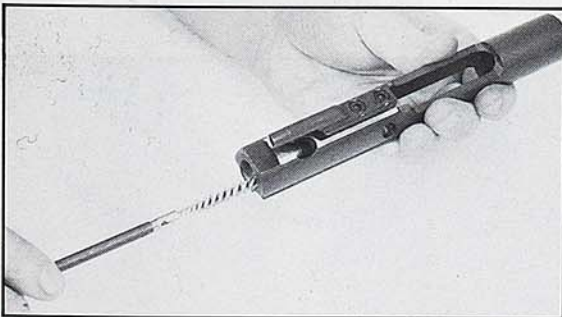
G. INSIDE BOLT CARRIER—FRONT.
