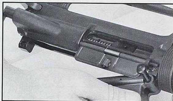
STEP 4. PULL PIVOT PIN OUT TO DETENT.
