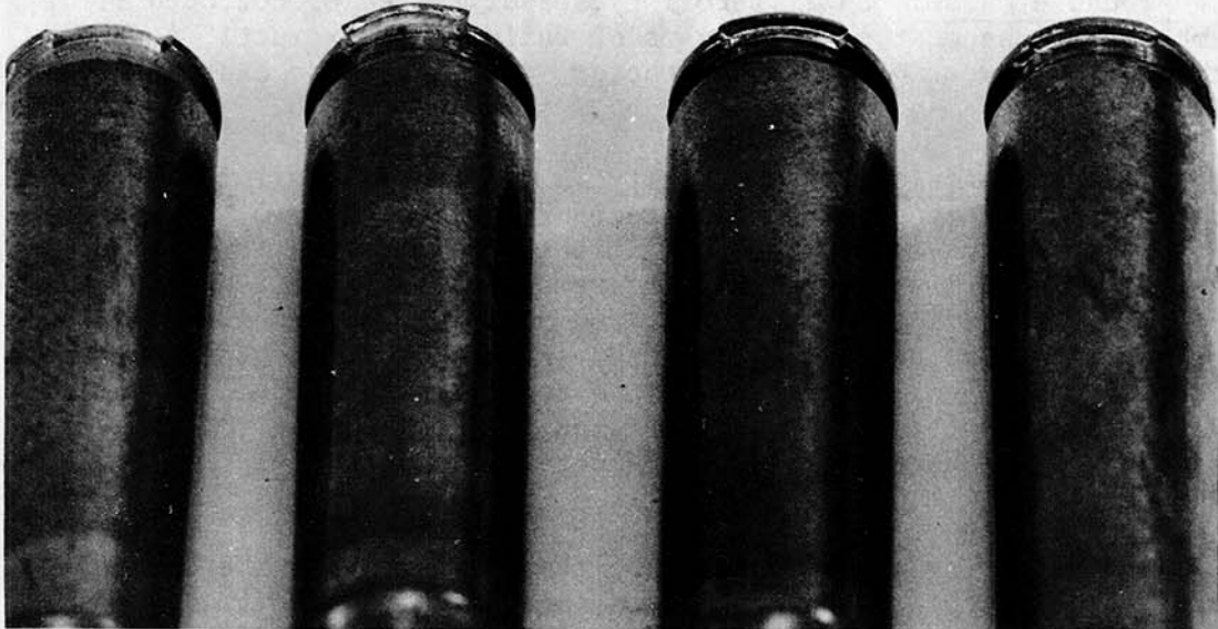
Figure I-7: Various Degrees of Rim Damage Which May Occur as a Result of a Failure to Extract (FX) Are Shown. (Cartridge rim at left is completely sheared, center two cartridges illustrate partial rim shears, while cartridge rim at right shows evidence of hard extraction. A normal extraction leaves only a faint and indistinct extractor mark on the cartridge case rim.)
