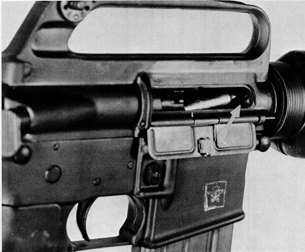
Figure I-9: Failure to Extract (FX) with a Live Round Jammed Against the Base of the Fired Case.
