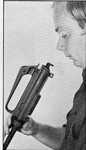
B. CHAMBER VISUAL INSPECTION
