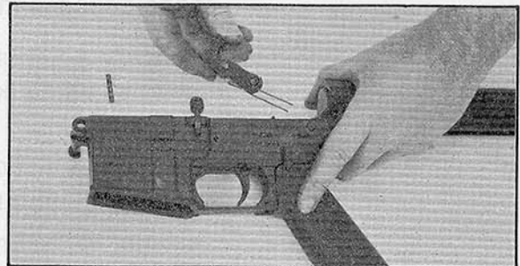
P. HAMMER REMOVAL
