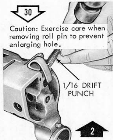
Remove/install roll pin.
