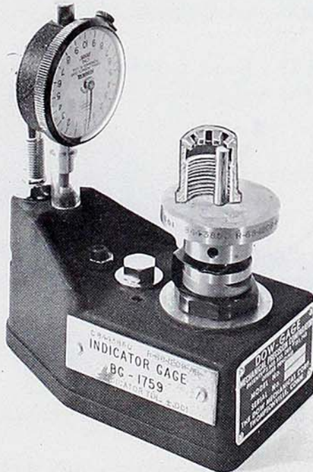
Figure 106. Zero Setting of Indicator Gage.
