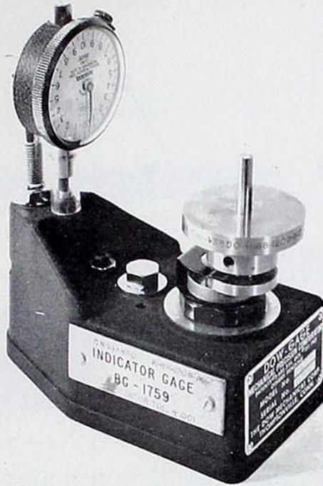
Figure 106. Zero Setting of Indicator Gage.
