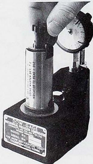
Figure 25. Insertion of Bolt into Indicator Gage.
