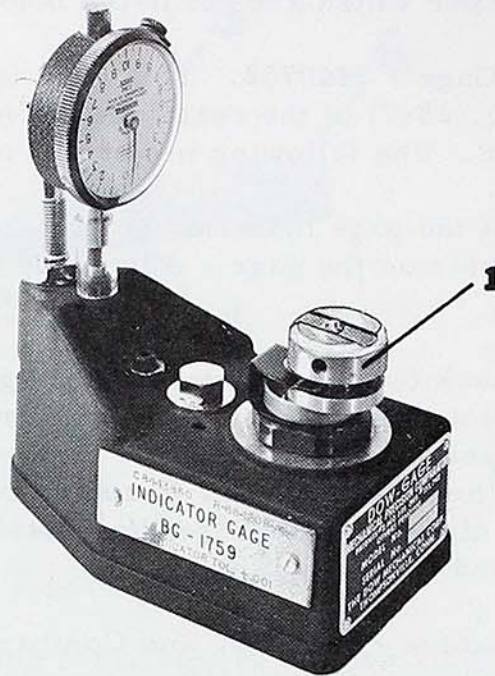
Figure 29. Zero Setting of Indicator Gage.
