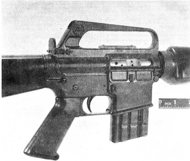
Figure 5: Modified AR15 Rifle. Note Riveted Cam Plate under Carrying Handle and Double Latch Charging Handle with Contact Pad at Rear End to Assist in Bolt Closing and Opening Operations.
