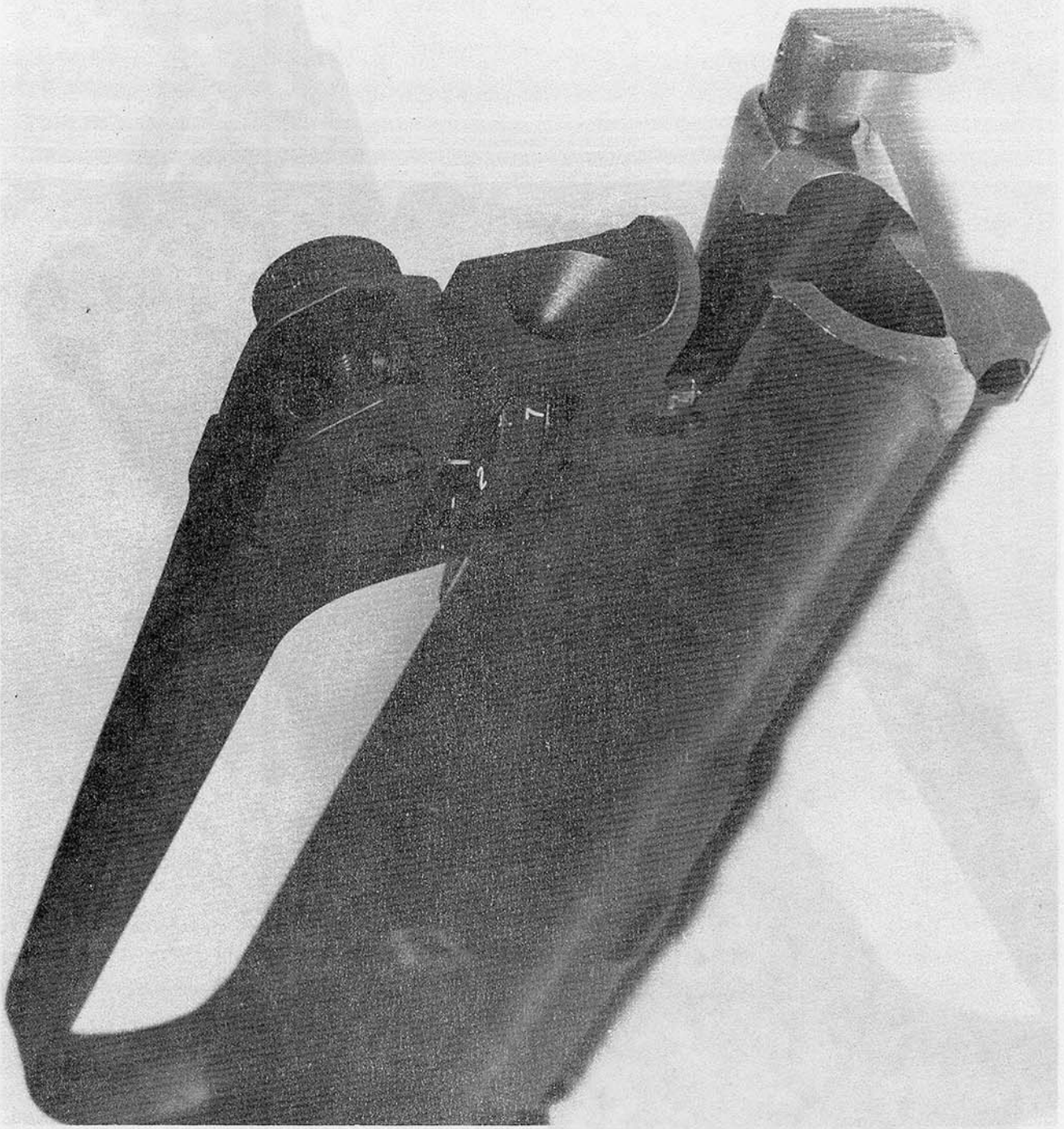
Figure 22. M16A1E1 upper receiver group left-top-rear view of adjustable rear sight in lowest position.
