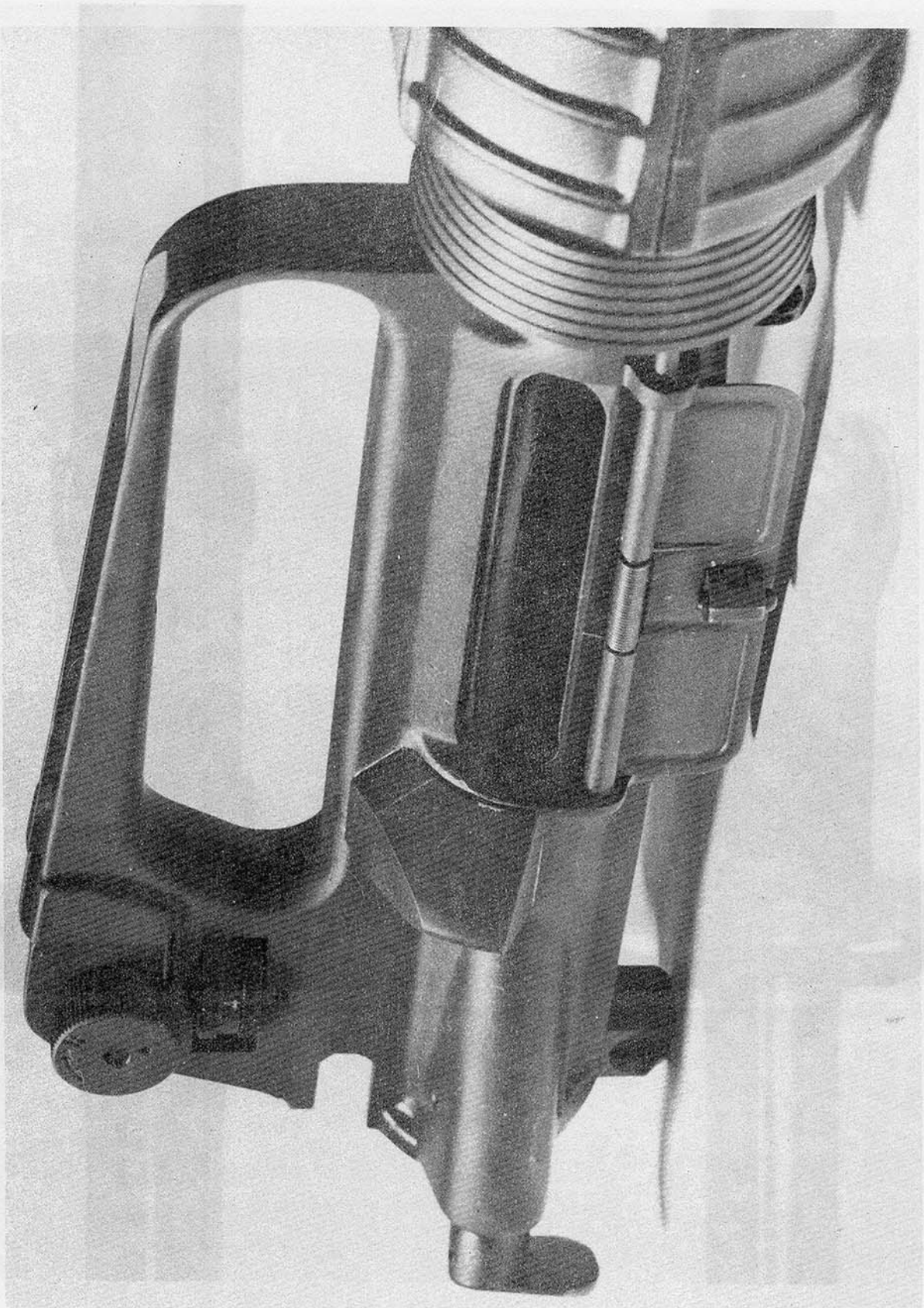
Figure 24. M16A1E1 upper receiver group, right frontal view showing details of spent case deflector and adjustable rear sight.
