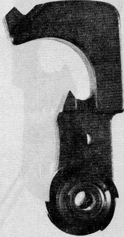
Figure 11. Hammer assembly for M16A1 (left) and M16A1E1.
