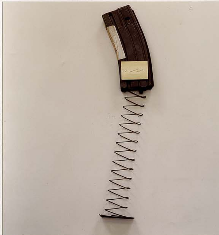
Figure 10 Colt magazine P2-4-2-1 with detached base plate after 1.5m Drop test at -46°C
