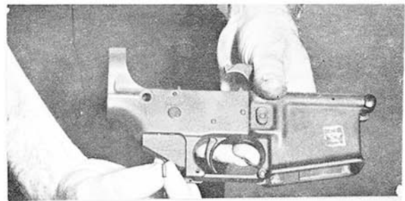
d. Detent Removed.
