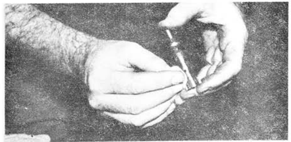
l. Wiping Outside Bolt.
