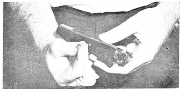
Step 2. Withdraw Firing Pin Retaining Pin.
