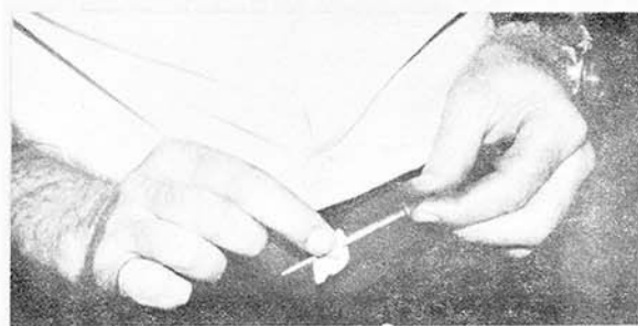
d. Wiping Firing Pin.
