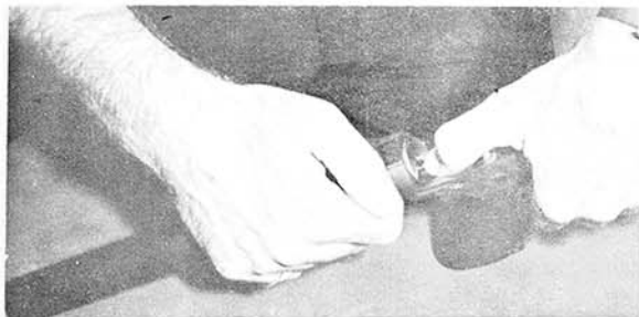
a. Buffer Retainer Depressed to Start Buffer Removal.
