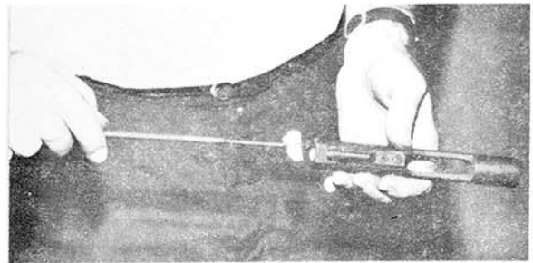
j. Wiping Inside Bolt Carrier - Front.
