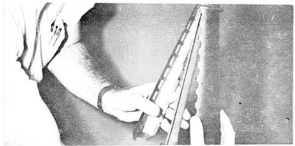
b. Handguards Released from Slipping.
