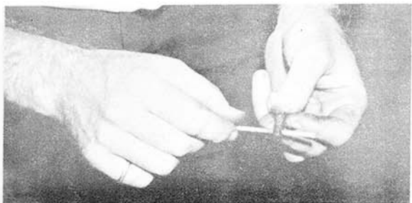
e. Wiping Inside Cam Pin.
