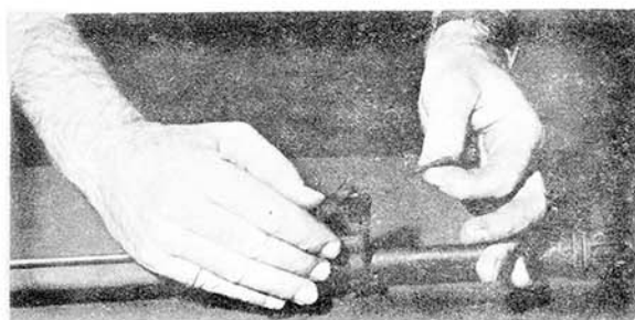
c. Front Sight Detent Removed.
