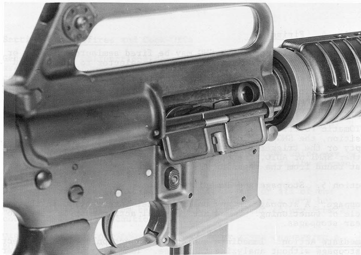
Figure 15A & 15B. SMG-Properly Loaded with a 20 Round Magazine, Charging Handle Locked Forward & Dust Cover Open. Bolt Open
