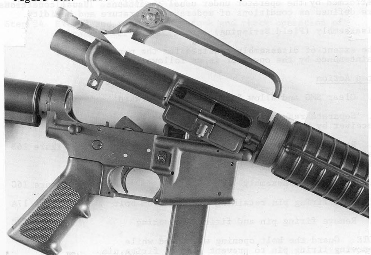
Figure 16B. Arrow shows charging handle being removed and the bolt becoming visible
