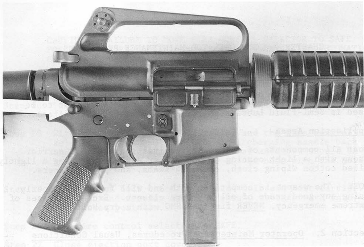
Figure 16A. Arrow shows rear take down pin. Push left to right.
