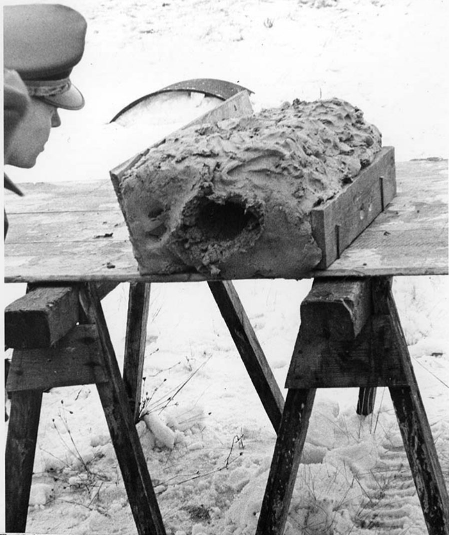
#7-This picture shows the effect when a 5.56 bullet is fired into heavy clay. The cavity was approx 5" dia X 6" deep.
