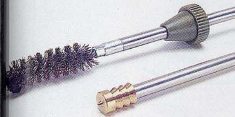
The basic tools of bore cleaning are rods with brushes or jag tips.
