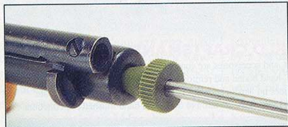
Here's how you use a bore guide to protect the muzzle crown.
