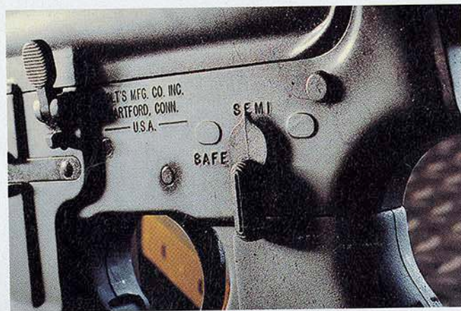
Right side of Colt M4 (above left) shows rear sight atop carry handle, forward bolt assist, magazine release. Left side of Colt M4 (above right) shows bolt release and "safe"/"semi" safety (fully automatic is available to military and law enforcement only), trigger. Below, butt stock can be extended.
