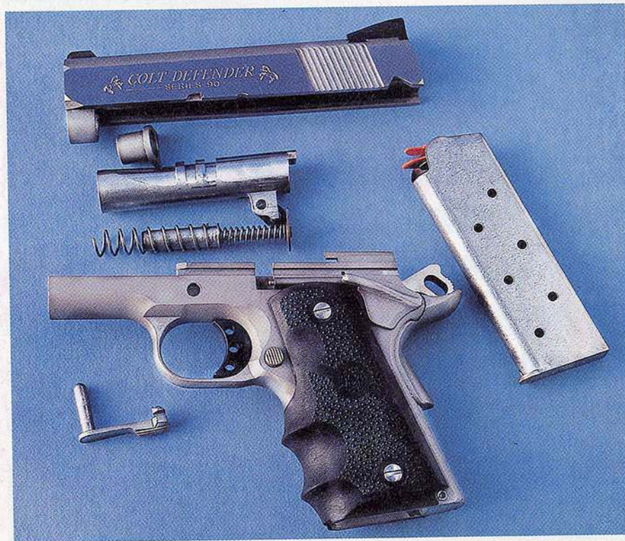
The Defender, disassembled. The flared barrel and dual recoil spring enhance performance.
