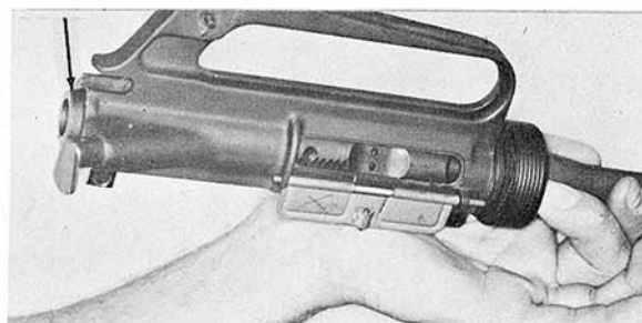
d. Proper Headspace Indication Bolt Will Not Go To Locked Position.
