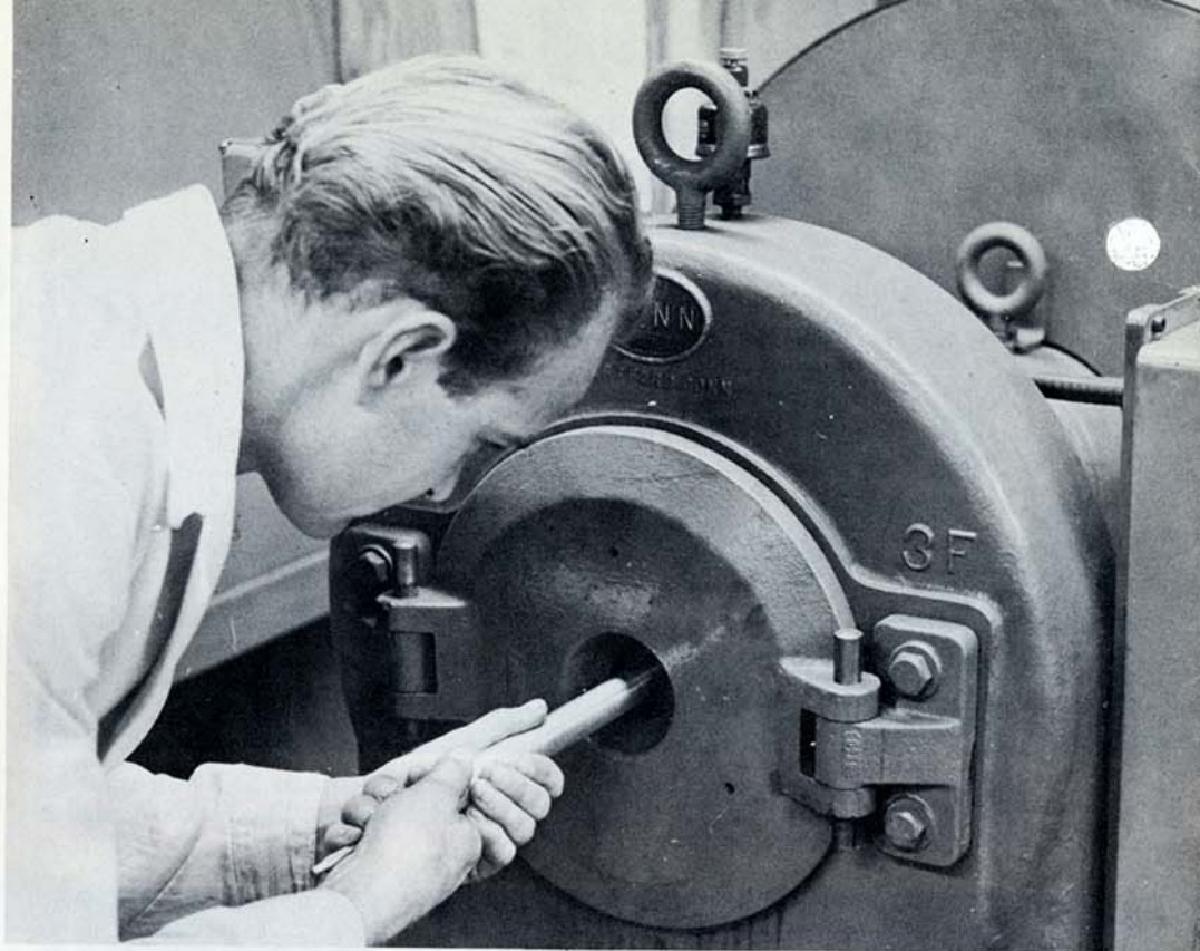
Swaging machine forms aluminum barrel jacket over stainless steel liner in fast operation for low-cost construction of erosion-resistant AR-10 barrels.
