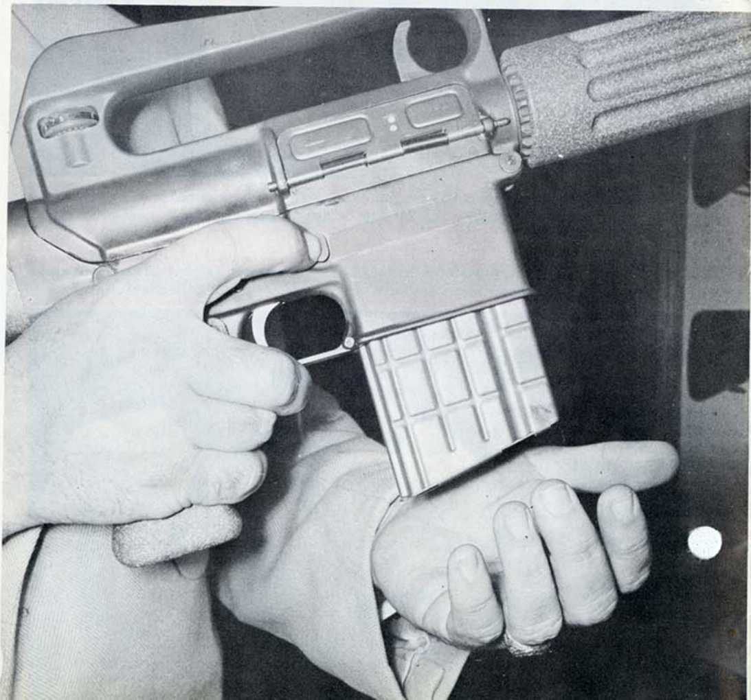
AR-10 breech is protected from dust and dirt since spring cover closes ejection port and strong waffle-creased clip is shrouded by frame.
