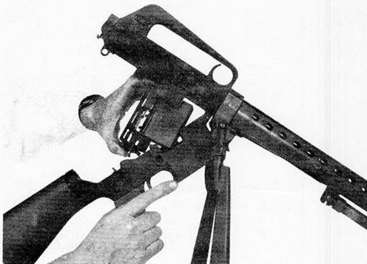
fig. 4 Method of Installing Belt Feed Mechanism
