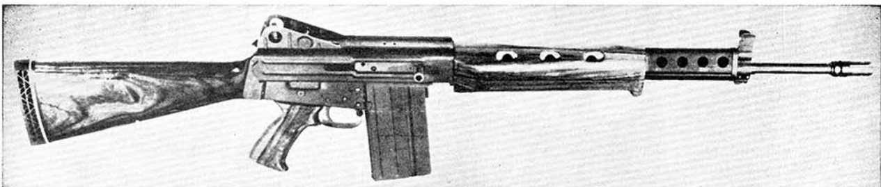
AR-16 (1959-1960) prototype rifle firing caliber 7.62 ammunition was designed as a low-cost version of the AR-10. Because of waning interest in a 7.62 rifle, the weapon was never produced in commercial quantities.
