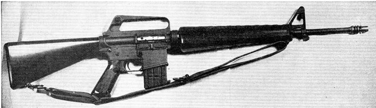
AR-15 (1956-1960) uses caliber 5.56-mm ammunition. Manufactured under license by Colt, the weapon has been issued as the M-16 to U.S. Forces. A nonautomatic modification is sold as a sporting rifle.
