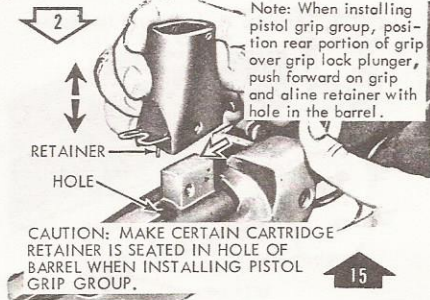
Remove/Install pistol grip group.
