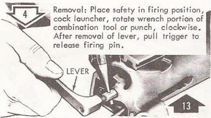
Remove/Install barrel group.
