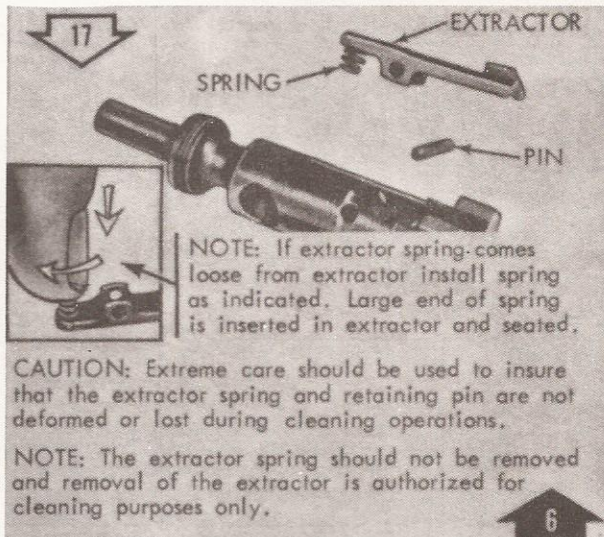
Remove/Install extractor and extractor spring.
