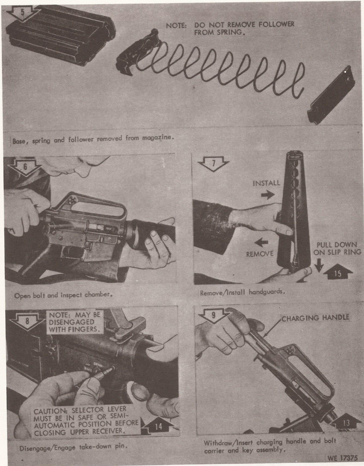
Figure 3-10. Disassembly/assembly of rifle. (2 of 5)
