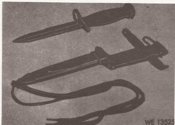
Figure 4-1. Bayonet-Knife, M7 and Bayonet-Knife Scabbard, M8A1.
