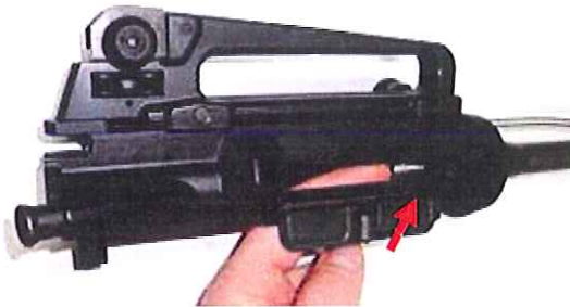
Step 1. Install the Headspace Gauge in Chamber.
