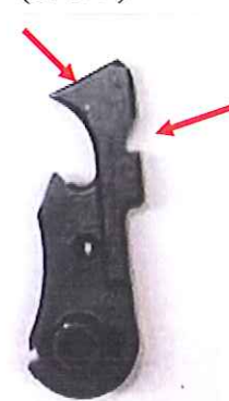
9mm Carbine (.170) Modified for Anti-Slam Fire on 9mm Bolt group. (62865)-.154 (63612)-.170
