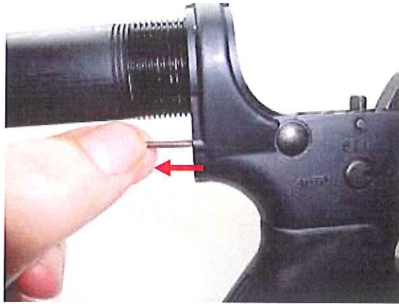
Step 6. Remove the takedown pin spring (61692).
