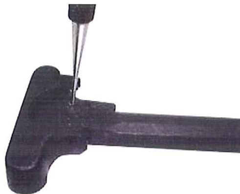
Step 1. With a 1/16 th inch punch, drive out the charging handle latch pin.
