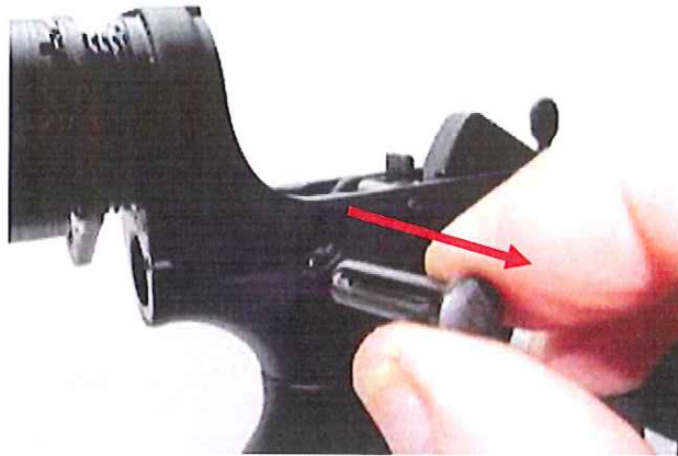
Step 7. Remove the rear takedown pin (61655) from the receiver.
