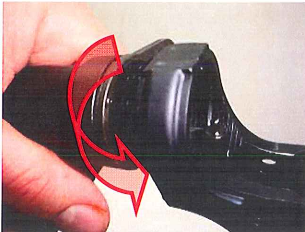
Step 8. While holding the buffer retainer in place, rotate the stock counter clockwise until it comes free of the receiver.
