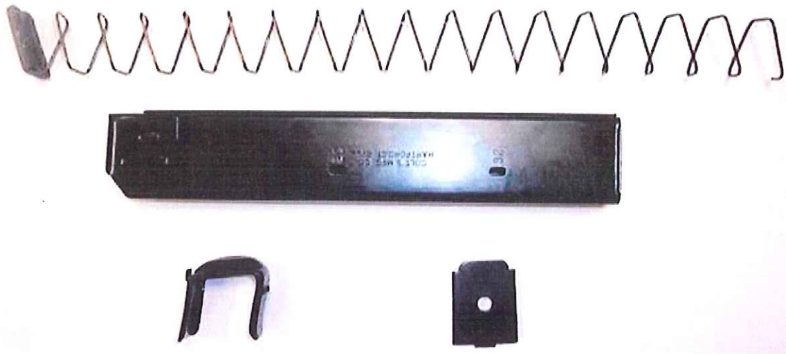
Step 3. Fully disassembled 9mm SMG magazine.
