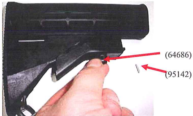
Step 2. Remove the nut. Hold nut and turn lock pin clockwise to remove nut.
