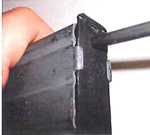
STEP 1. Floor plate removal.
