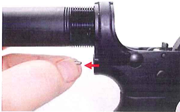
Step 7. Remove takedown pin detent (61698).
