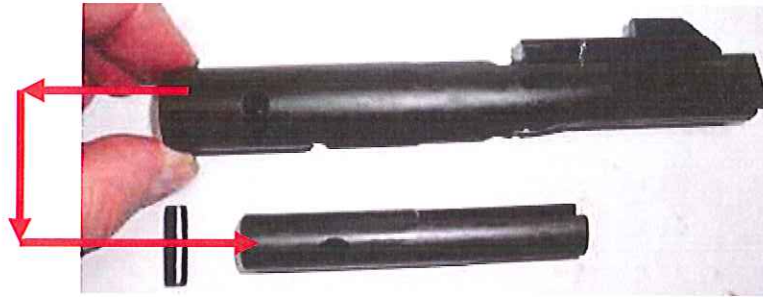
Step 4. Remove the plug (62807)
