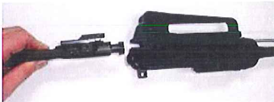
Step 3. Install Bolt Carrier Group.
