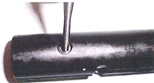
Step 3. DO NOT REMOVE UNLESS NECCESARY FOR REPAIR!! With a 3/16-inch drift punch, remove the spirol pin (95222).
